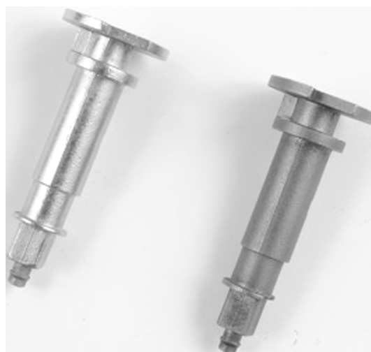
Figure 10. Stainless steel 316 polished (left) and unpolished (right).
