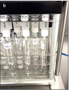
Figure 2-7 Automated extraction system, Biotage® PRESSURE+
