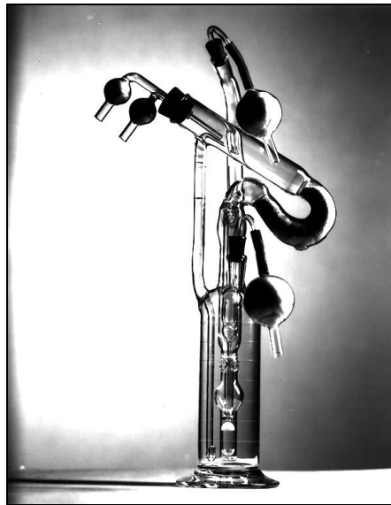
Figure 2.11 The first organ perfusion pump developed by Carrel and Lindbergh (101).
