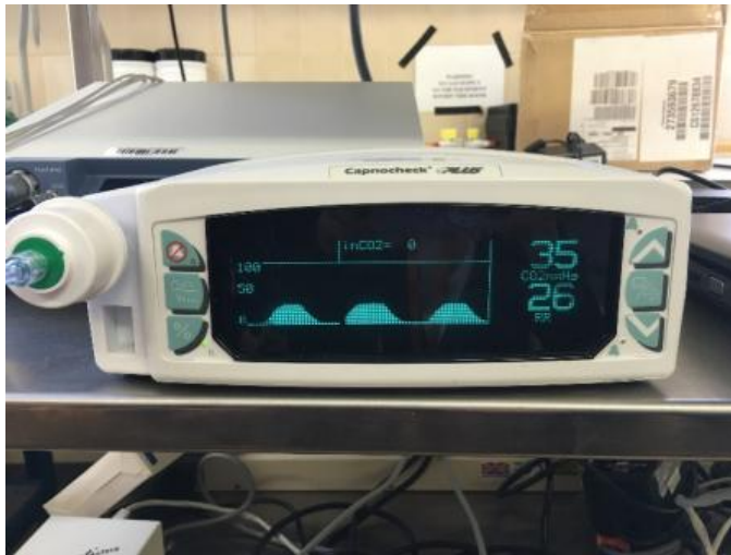
Figure 4.2 Capnograph showing breath-by-breath waveforms of ETCO 2 .
