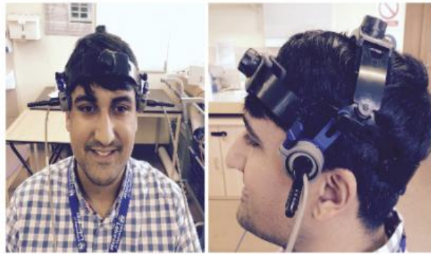
Figure 1 and 2, Head-frame with ultrasound probes
