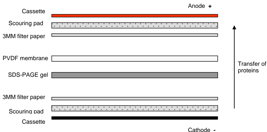
Figure 2.2. Apparatus assembly used for electro-blotting of proteins from SDS-PAGE gels to PVDF membranes.
