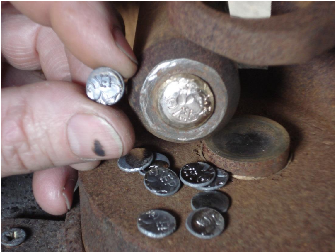
Figure 2.47: Replica coins after minting, with the upper die and (blank) lower die lying alongside
