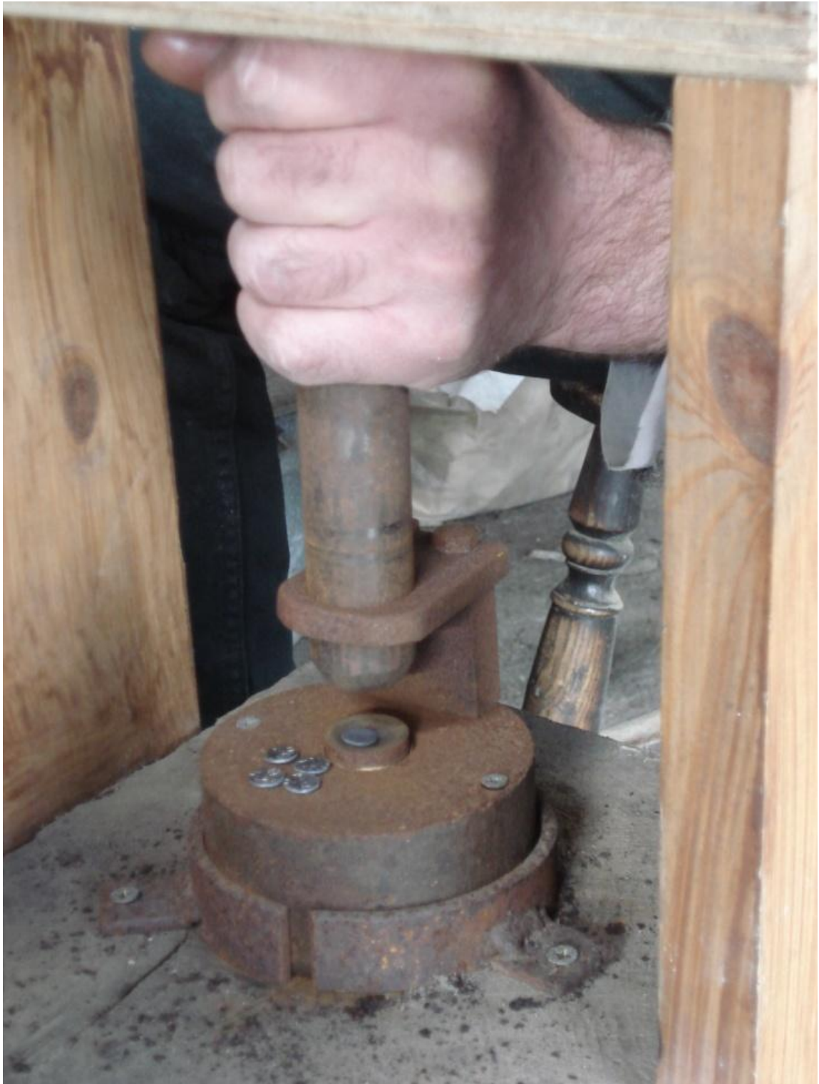
Figure 2.46: The die-support arrangement used by Neil Burrige
