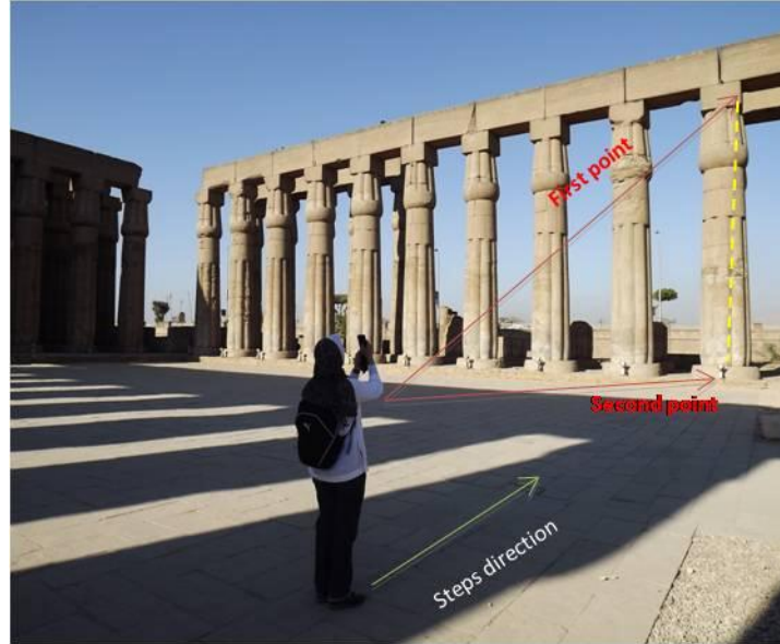
Figure 3-11: The measurements to obtain Temple heights using SpectaRuler iPhone (Luxor Temple Dec. 2011)
