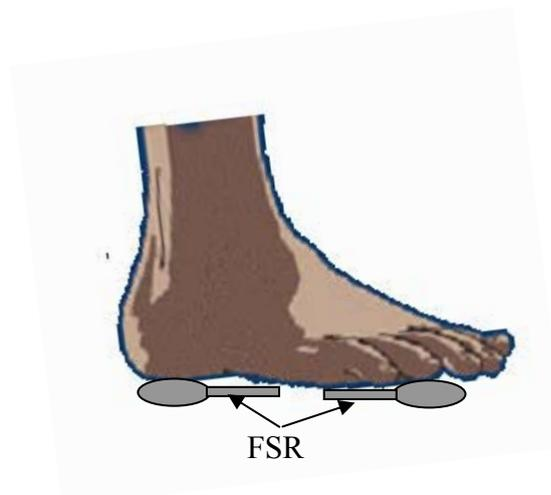
**Figure (5.2)** - Force sensitive resistor placed under the heel and the toe
