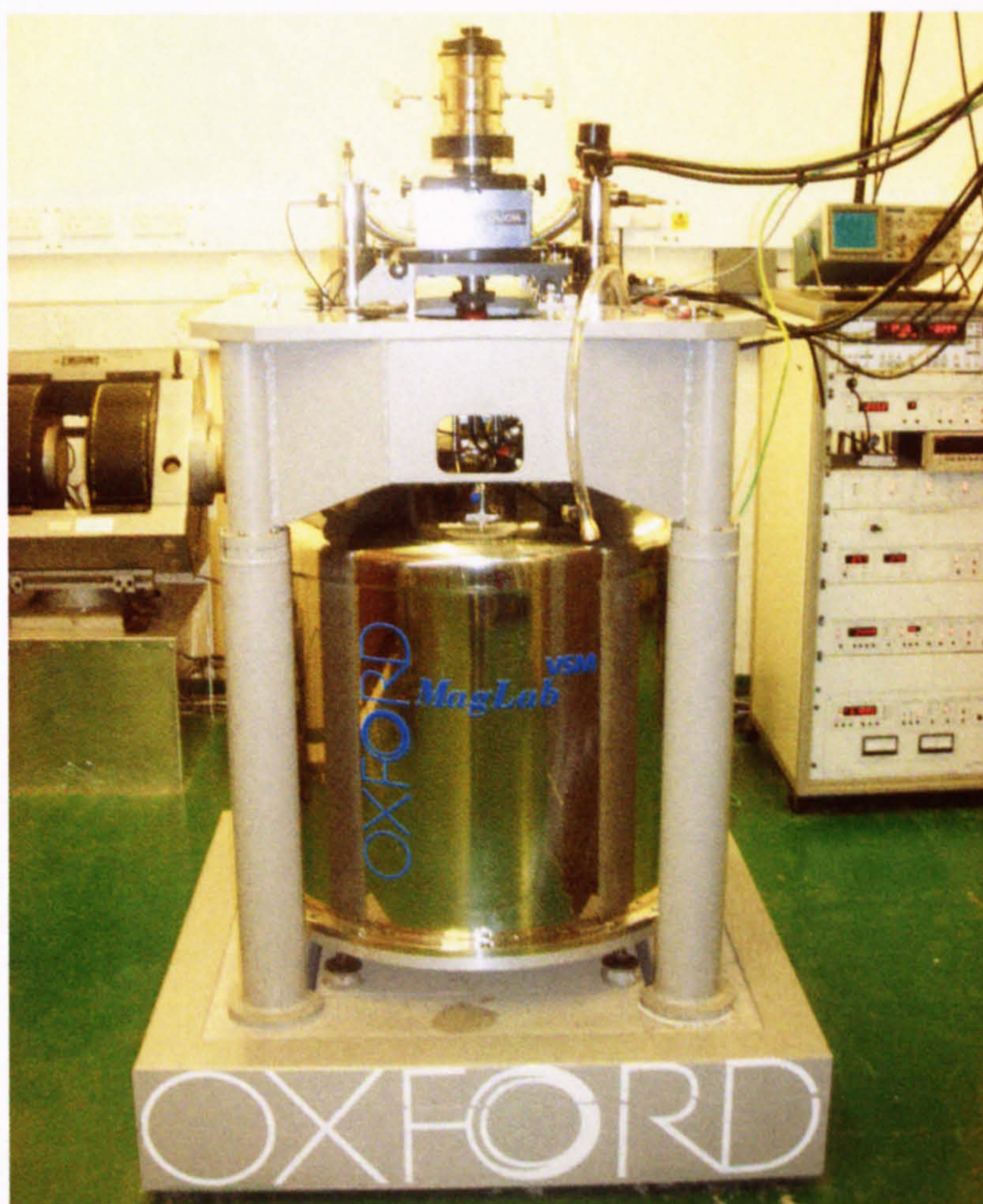
Figure 3.14 University of Leicester 9T magnetometer
