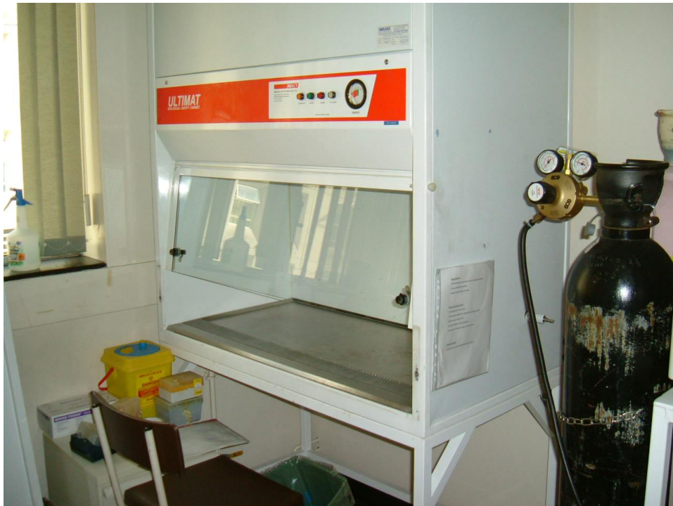
Figure 2.1: Flow cabinet used for culture tissue and preparation. Laminar flow of air prevents contamination of tissue specimens by bacteria and fungi. When not in use, ultraviolet light maintains sterility. All instruments introduced into the cabinet are sprayed with alcohol to sterilise
