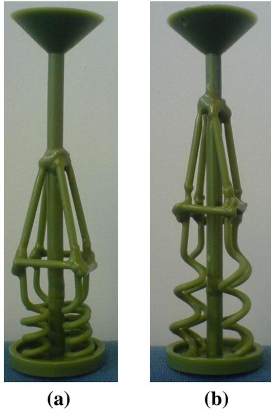
**Figure 4.26** Wax moulds with different spiral take-off angles ( $\theta$ ) of: (a)  $28^\circ$  and (b)  $50^\circ$
