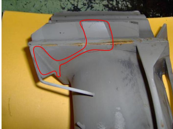
**Figure 5.8** Formation of stray grains at the platform region in IN792 turbine blades (Courtesy of Rolls-Royce Plc.)
