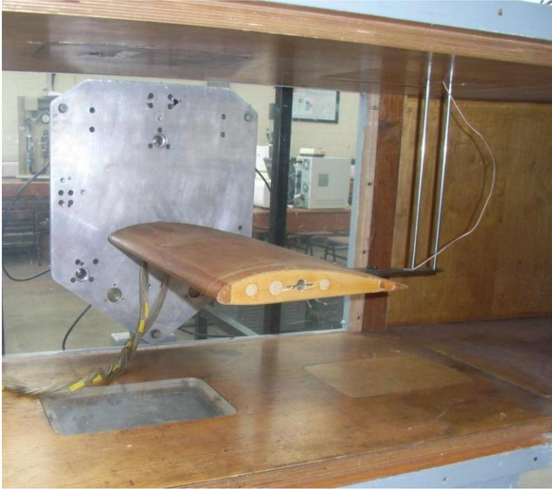
*Fig. 5.* Tests were carried out with a model aerofoil to determine whether variations in the data were a result of underlying error in the balance and software or a result of turbulent flow around the models. The aerofoil was a shape well suited to producing laminar flow and the same length as the models.
