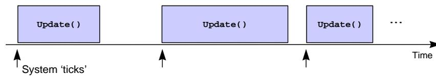
Figure 18: One advantage of the interrupt-driven approach is that the tasks will not normally suffer from “jitter” in their start times.
