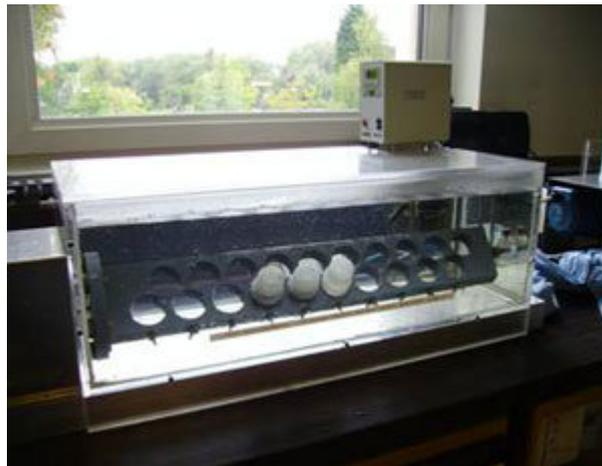
**Figure 3.9:** Apparatus used for PBET extractions. Image courtesy of the British Geological Survey.
