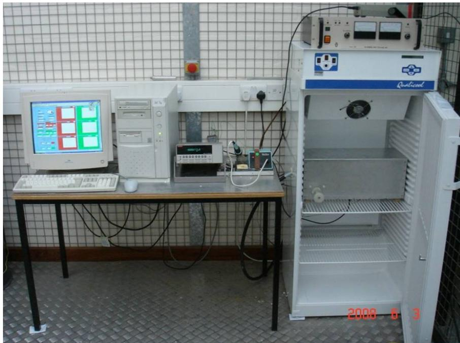
Figure 3.24 Charging/discharging experiment system with picoammeter
