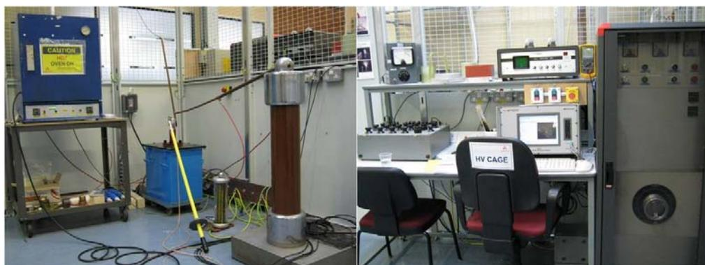
Figure 5.17 Schering bridge system setup. High voltage part in the left photo and low voltage control part in the right photo.
