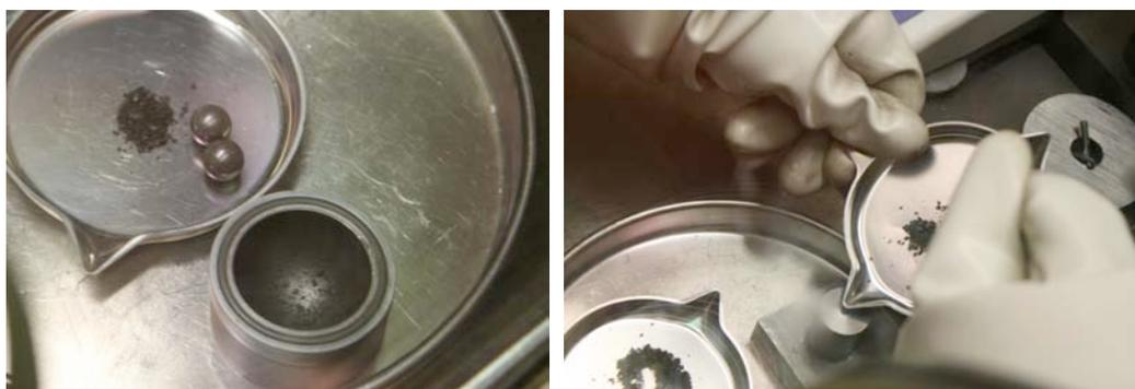
**Figure 6.2:** (*Left*) Post ball mill mixing of sample batch L1. (*Right*) Pouring W-AmO<sub>2</sub> mixture into die.
