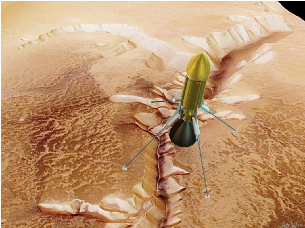
**Figure 7.10:** Author’s Illustration of a Mars Hopper at the apogee of its “hop”. Attitude control and ground-looking instrumentation assess and select potential landing sites prior to activation of a descent control firing of the heat capacitive RTR.
