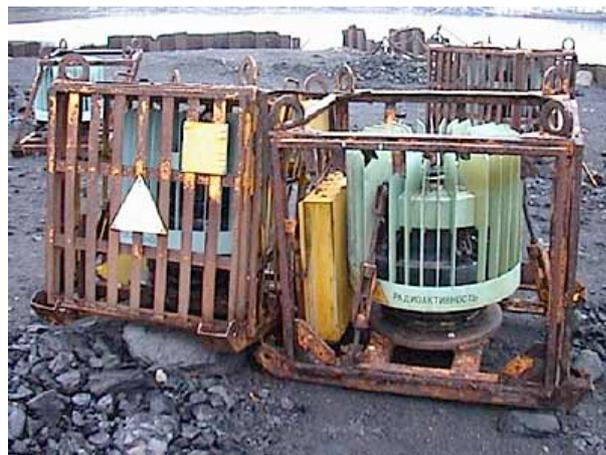
**Figure 2.1:** Disused  $^{90}\text{Sr}$  fuelled Beta-M RTGs used for remote power operations. Image courtesy of Finnmark Region Government.
