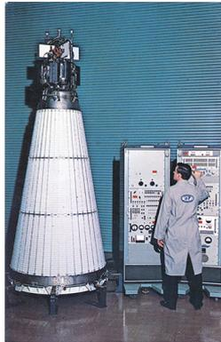
**Figure 2.9:** Photograph of the SNAP-10A during ground based testing. Image courtesy of NASA.
