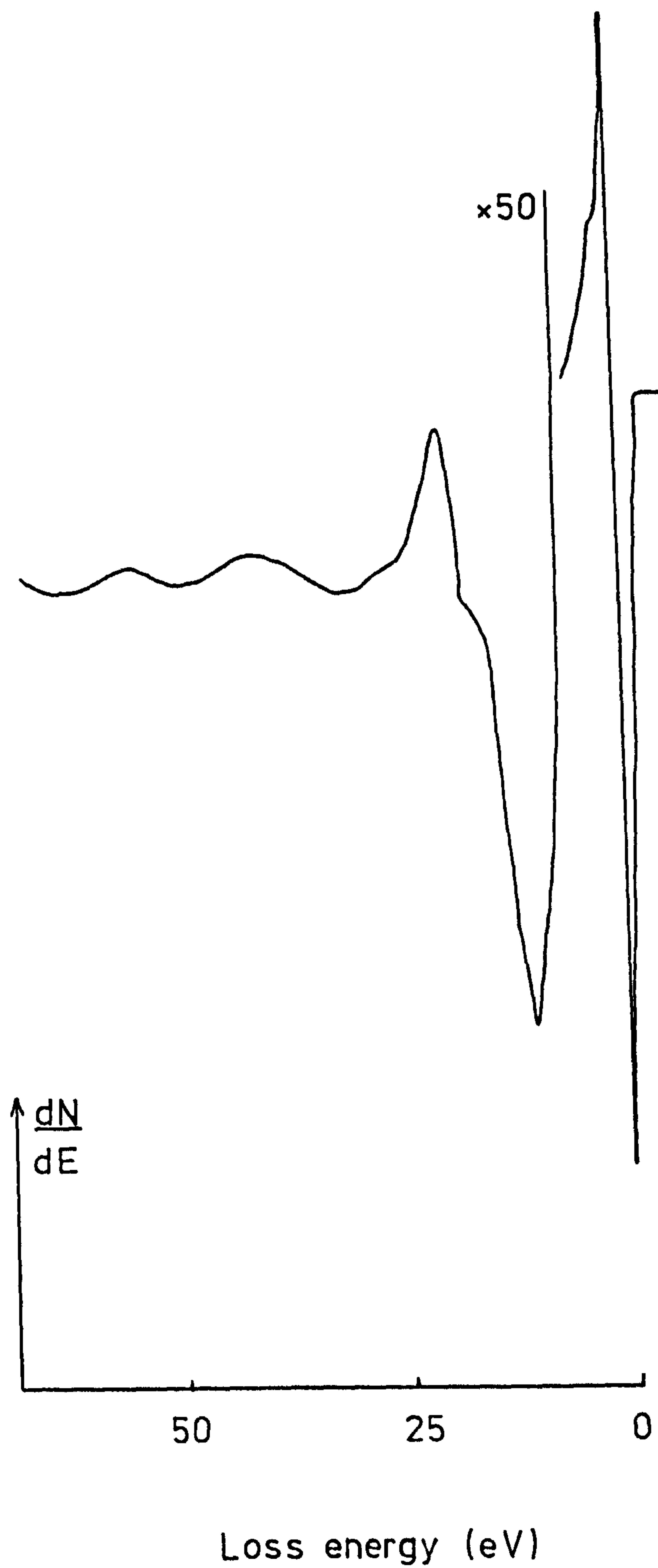
Figure 5.23. Electron energy loss spectrum with glancing-incidence electron gun.
