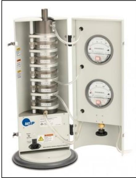
**Figure 4.1: Ten-stage rotating MOUDI for the collection and particle size determination of bioaerosols**
