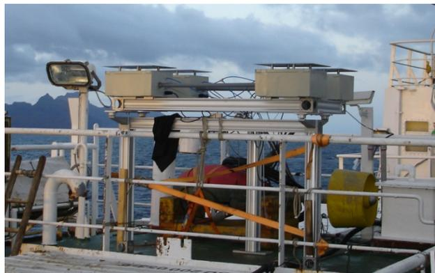
Figure 4.5. BBCEAS instrument cavity mounted on the gantry on the deck of RSS Discovery. Two BBCEAS cavities are shown in tandem; Leicester I<sub>2</sub> detector and Cambridge IO detector. The BBCEAS is shown in a background ( $I_0(\lambda)$ ) measurement mode in which a length of plastic tubing is inserted to enclose the light path and a flow of nitrogen gas passed into the enclosure to expel ambient air.
