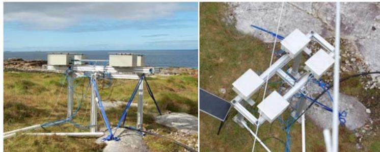
Figure 5.6 BBCEAS instrument cavity mounted on gantry at Mace Head. Two BBCEAS cavity instruments set up in tandem: the Leicester I<sub>2</sub> detector and Cambridge IO detector. Pictures taken by the author from the tower between and above the shore side cottage laboratories at Mace Head.
