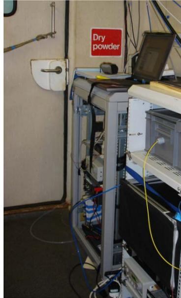
Figure 3.24 The 19" rack housing the electronic components of the BBCEAS instrument: in situ onboard RSS discovery during D319.
