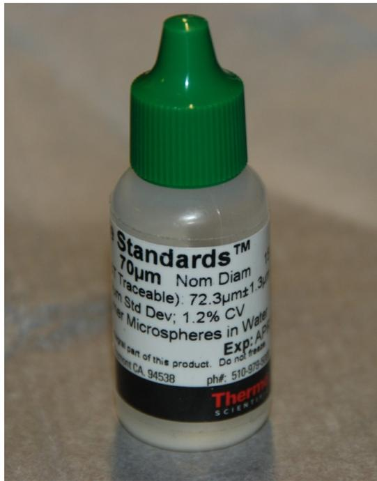
Figure 5.7: The Microsphere particles used for validation purposes.
