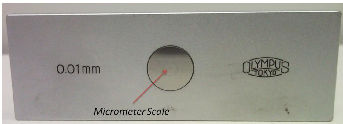
Figure 5.2: The objective Micrometer Plate.
