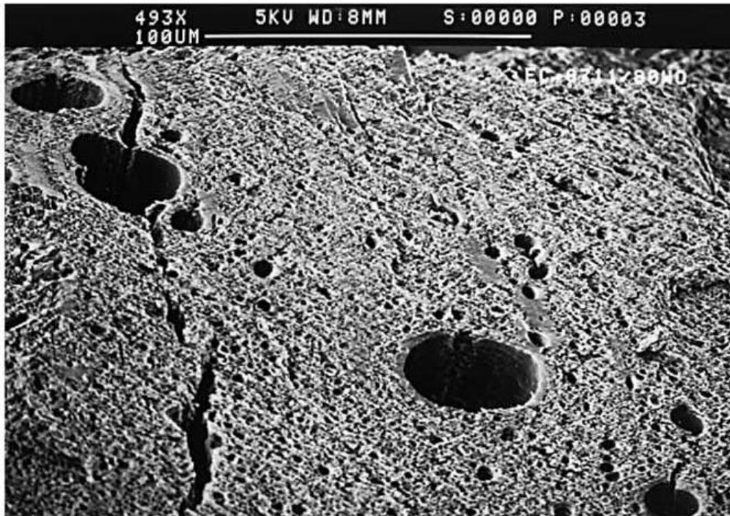
**Figure 2.3.3** Cross-section image of a PLLA implant after 80 weeks (Gutwald *et al.*, 2002).
