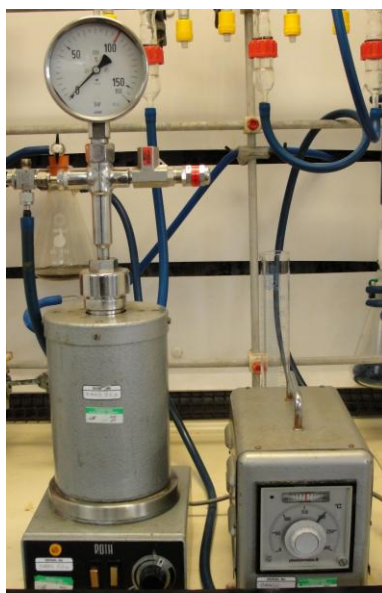
Figure 45: High pressure apparatus used for the rhodium-catalysed Fischer indole reaction.
