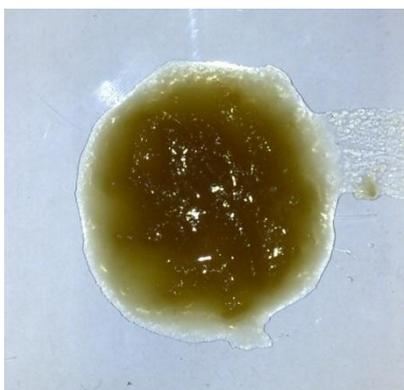
*Figure 8.1: Photograph of the Polymerized Ageing Product after 84 Days at 150°C*
