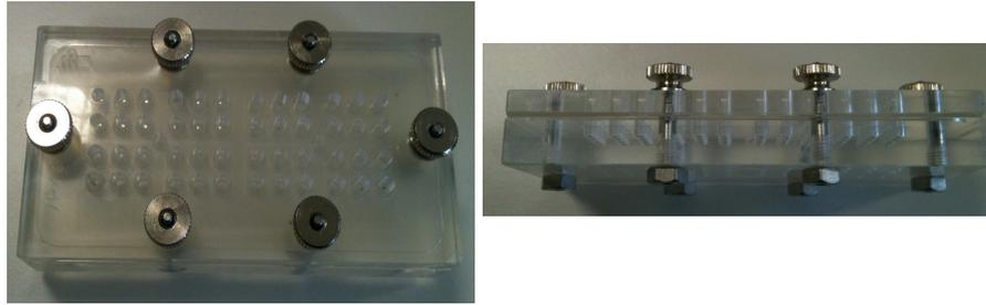
**Figure 2.4. Photograph of the 48 well Boyden chamber from above (left) and the side (right).**
