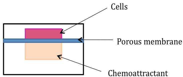
**Figure 2.5. Diagram demonstrating the set up of one well of the Boyden chamber**
