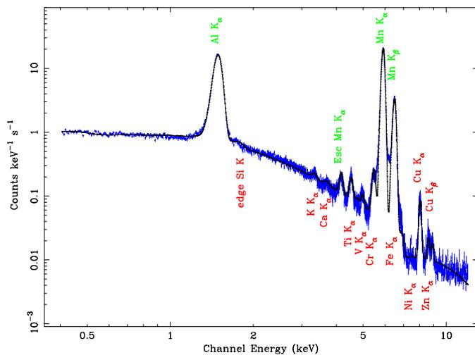
**Fig. 6.** Calibration spectrum with the internal radioactive source including the background with the filter wheel in closed position. The continuous background below the Mn lines arises mainly from photoelectrons stimulated from the  $^{55}\text{Fe}$  source in the Al target. The iron  $\text{K}\alpha$  line between  $\text{MnK}\alpha$  and  $\text{MnK}\beta$  is not resolved
