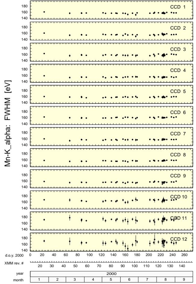
**Fig. 8.** The full width at half maximum of the internal calibration source. The larger errors in CCD's 10, 11 and 12 are due to the inhomogeneous focal plane illumination resulting in a reduced count rate
