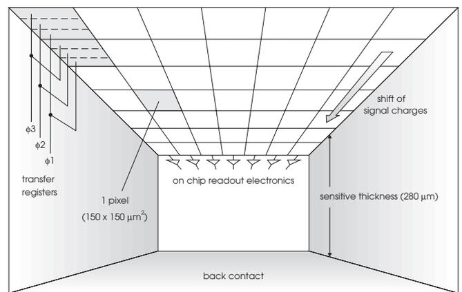
**Fig. 1.** Inside the pn-CCD. The X-rays hit the device from the backside (bottom). The charges are collected in the electron potential minimum 10  $\mu\text{m}$  from the surface having the pixel structure. After integration, they are transferred to the on-chip amplifier. Each CCD column is terminated by an on-chip JFET amplifier
