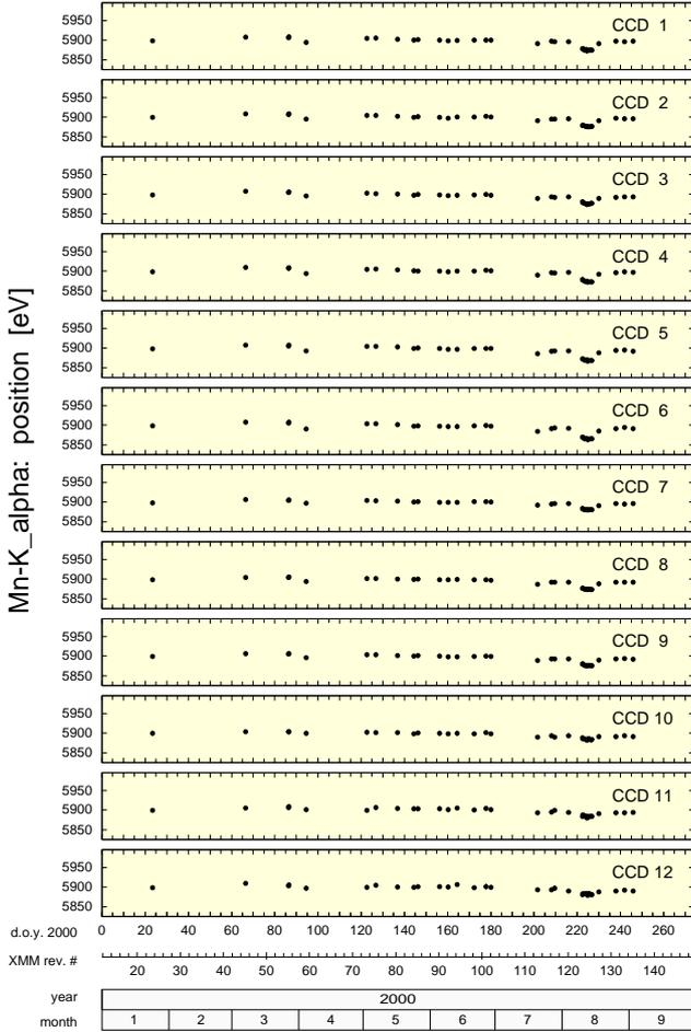
**Fig. 7.** Longterm stability of the pn-EPIC camera system monitored with the internal calibration source. Within a precision of 5 eV no CTE related peak shifts were observed, given nominal operation temperatures in the pn-CCD camera system
