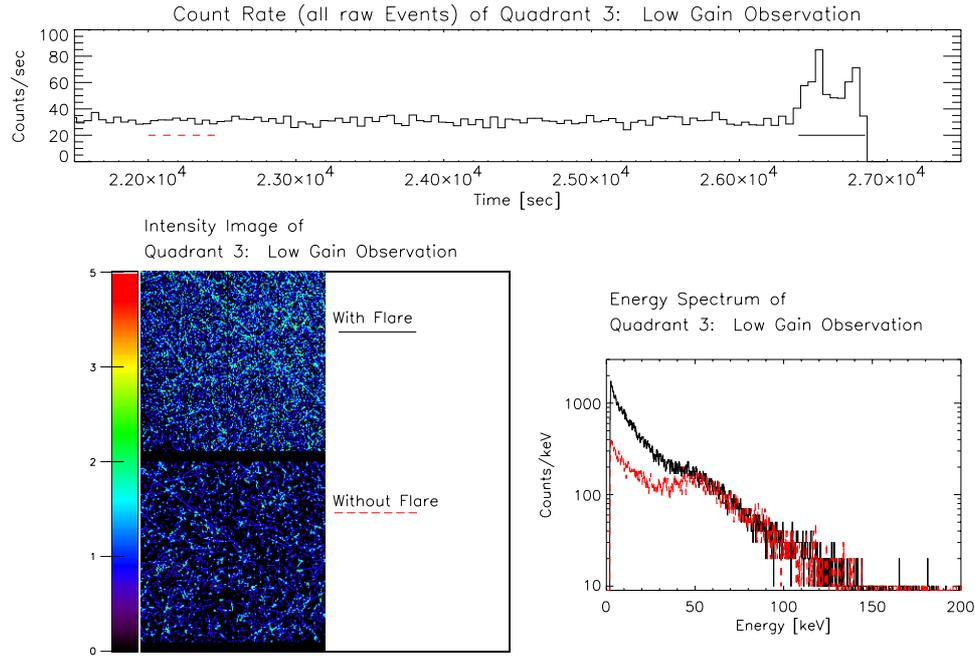
**Fig. 9.** Measured background spectra (thick filter) with a reduced gain (factor 20) during normal background, mainly mips (red line) and during a “soft proton flare” (black line). The upper panel shows the “light curve” of the observation with an increased background in the last 500 s. The lower left picture shows the event pattern of the high and low background measurements. The lower right diagram shows the difference in energy deposition for the low and high background events
