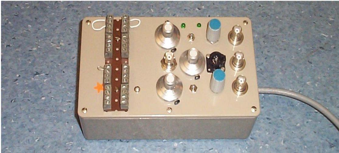
*Figure 3-38: Photograph of the 'Input Pod'. The Potentiometers are used to calibrate the signal to be measured to fit the full scale range of the data acquisition system.*
