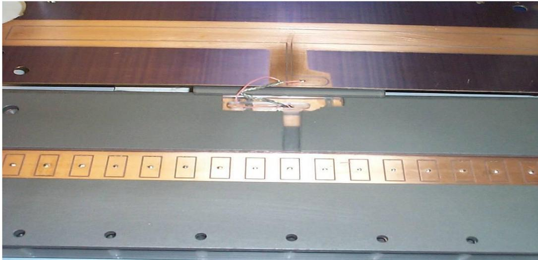
*Figure 3-16: The high tension plate, 5mm spacer and collecting plate ready for final assembly. The electrically conductive paint can be clearly seen on the spacer.*
