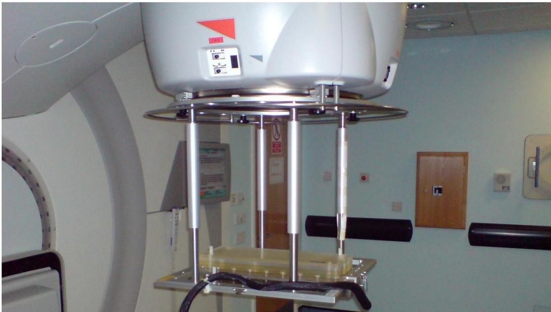
*Figure 3-18: The completed array fitted the accelerator radiation head accessory ring using the commercial holding device, with the required build up secured by 2 of the 4 threaded studs, ready to measure rotational beams.*
