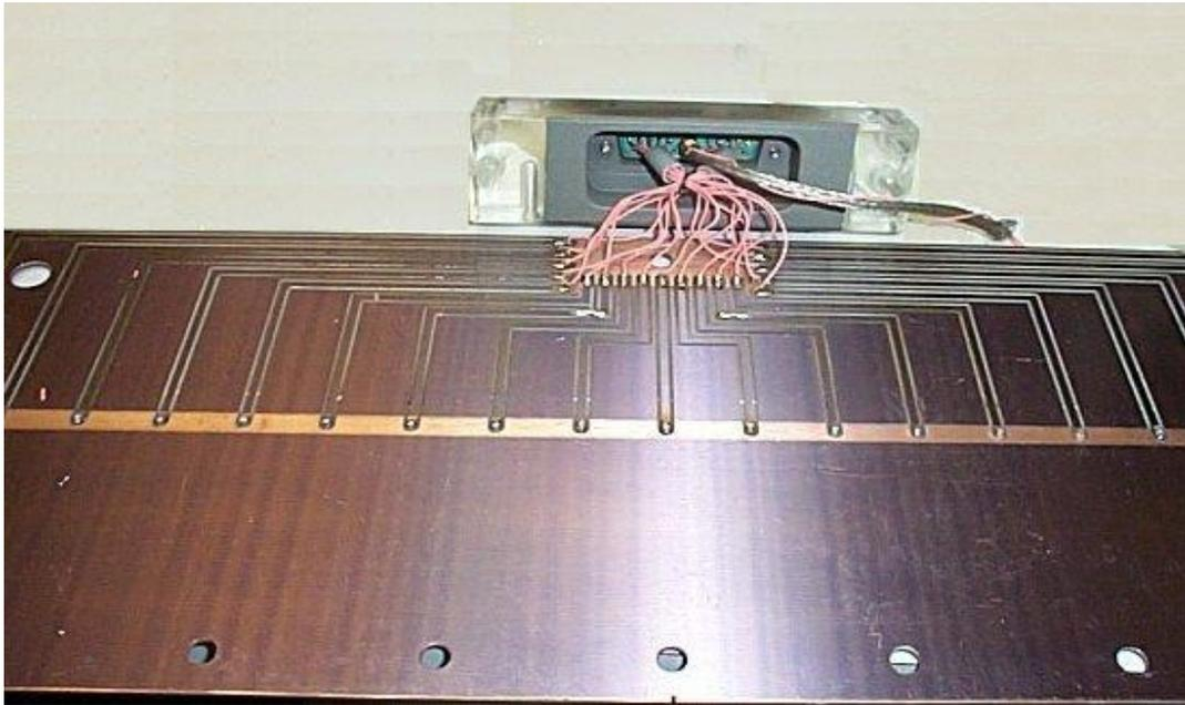
*Figure 10-7: External connector wiring (PTFE insulated) showing the signal tracks connected to the pins and the central coax connection in place ready to connect the star ground point and high tension supply.*
