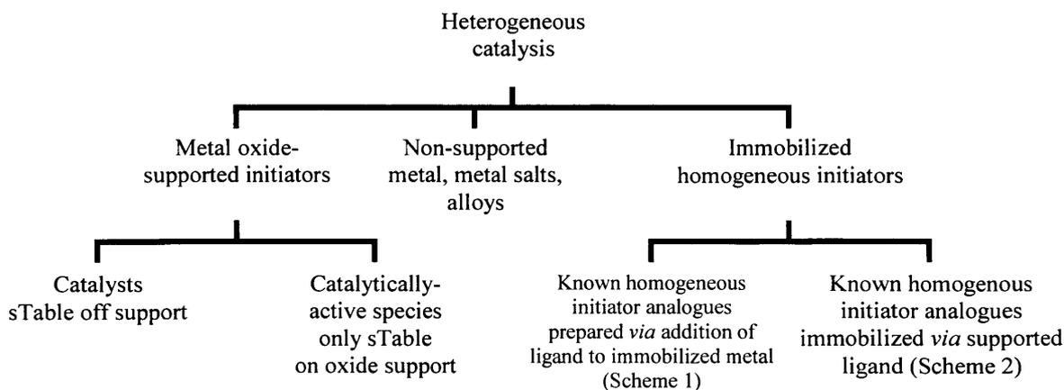
Figure 1 An overview of heterogeneous catalysis
