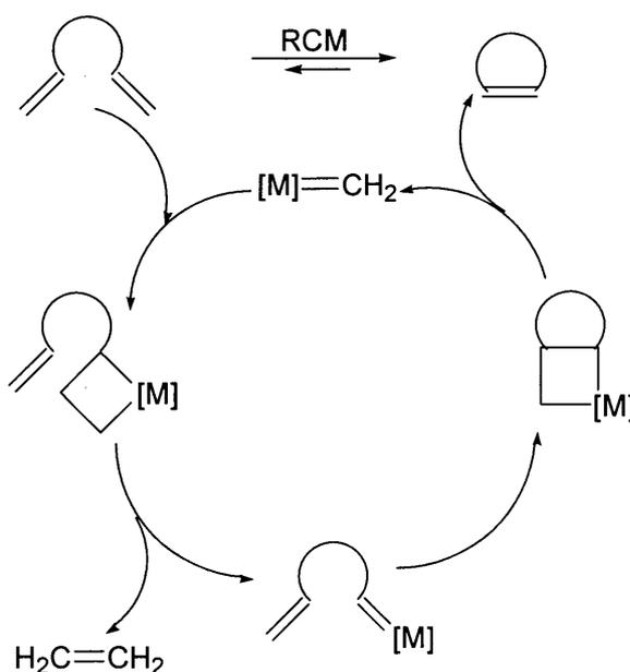
Figure 17 General mechanism for RCM reactions
