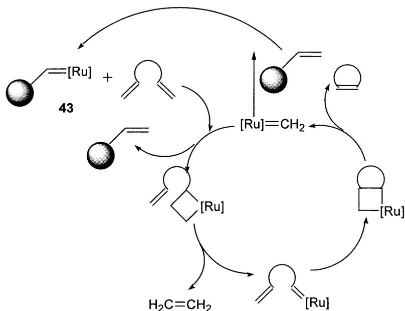
Figure 19 Supported Grubbs' initiator using the "Boomerang" effect
