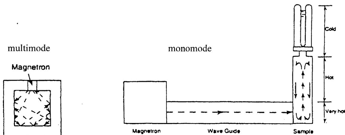
**Figure 7 Principle of multimode and monomode microwave**
