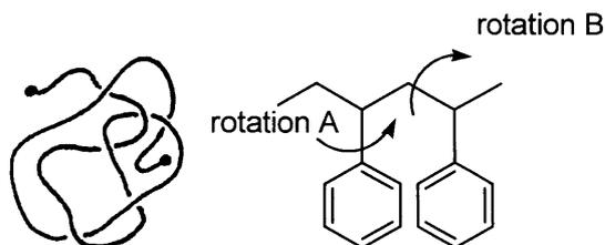
Figure 4 Linear polymer network and their rotations permitted in function of the temperature
