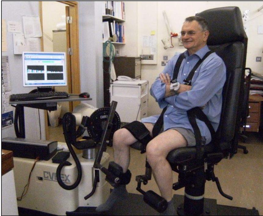
**Figure 4.2 – Subject positioning on the Isokinetic dynamometer**
