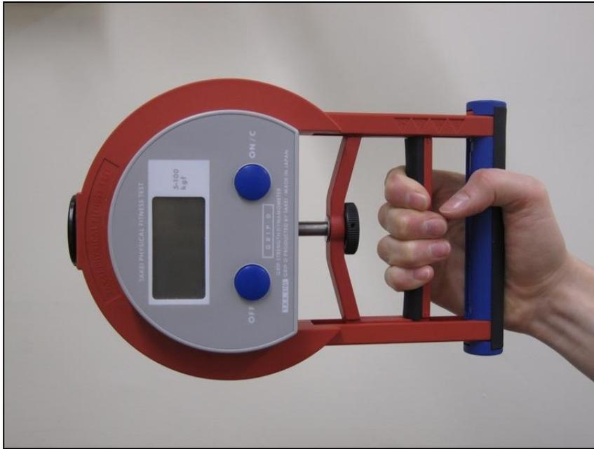
**Figure 3.2 – Handgrip Dynamometer**
