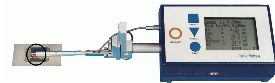
**Figure 2.9.** Photograph of a Silver Surtronic 3+ profilometer, stylus is circled in black.
