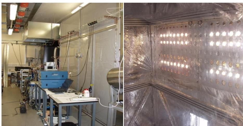
**Figure 18.** The Aerosol chamber at Manchester. The outer housing with the Leicester CIR-TOF-MS connected to the inlet (left) and inside the chamber with 18m<sup>3</sup> teflon bag and the arc xenon lamp with the bank of halogen lights (right)
