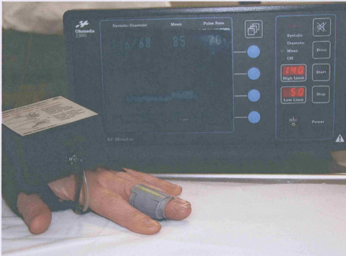
Figure 1:11 Finapres™ 2300, Ohmeda for non-invasive estimation of finger arterial BP
