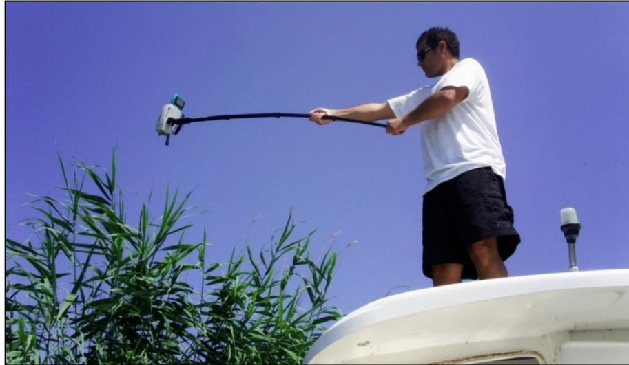
*Figure 3.2: Photograph illustrating the setup for collecting canopy field measurements from the waterward side of the reed bed with the aid of a motorboat at Bozsai bay in Lake Balaton, Hungary. The spectroradiometer is attached vertically at the end of a pole and is pointing downwards at the time of data acquisition.*
