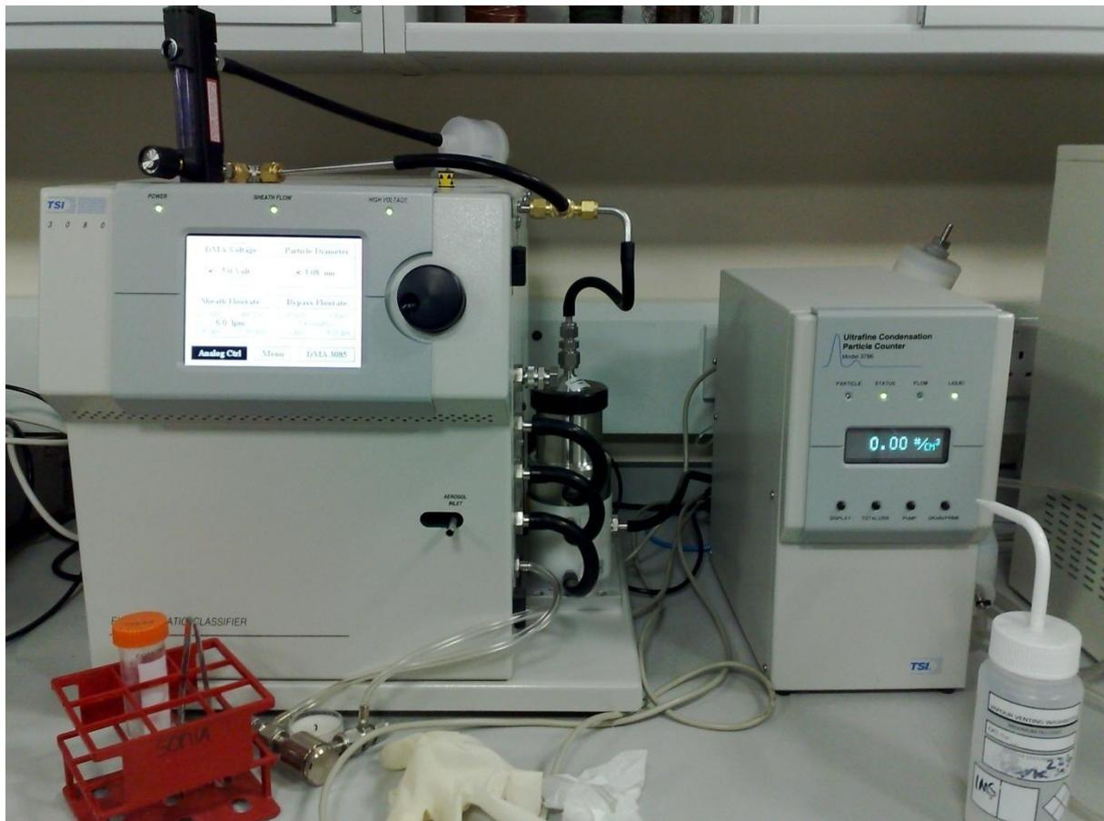
**Figure 2.13:** Photograph of Scanning Mobility Particle Sizer. Particle size was measured in a nitrogen gas stream using a TSI Scanning Mobility Particle Sizer.
