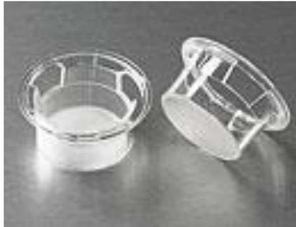
**Figure 2.5:** Transparent (when wet), collagen-treated PTFE membrane ( $3.0\mu\text{m}$ ), 6 well 24.5mm Transwell-COL insert are used for exposure studies. (Taken from Corning website).
