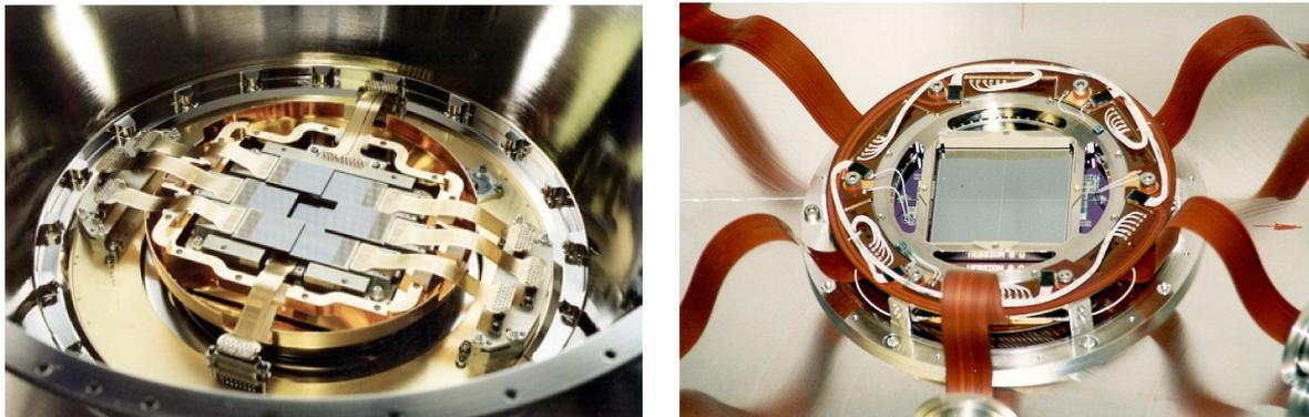
Figure 2.3: One of the MOS detectors (left) and the pn detector (right). Images taken from <http://xmm.esac.esa.int/> and courtesy of Leicester University, University of Birmingham, CEA Saclay Service d'Astrophysique, MPI-semiconductor laboratory, MPE, Astronomisches Institut Tübingen, Germany and ESA.
