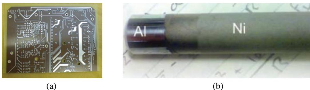
**Figure 1.13 :** (a) Immersion silver coating on multitrack circuit board from 1:2  $\text{ChCl}:\text{EG}$ <sup>97</sup> (b) Photograph of electrolytically deposited Ni from aqueous Watt nickel bath on immersion plated Cu Al rod<sup>97</sup>
