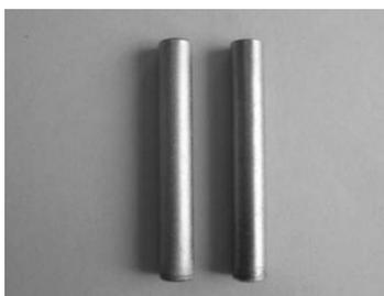
**Figure 1.10 :** Photographs of potentiostatic deposition of hard chromium film (25-30  $\mu\text{m}$ ) from  $\text{ChCl}:\text{CrCl}_3\cdot\text{H}_2\text{O}$  on XC38 steel (left) and SS304 (right)<sup>97</sup>
