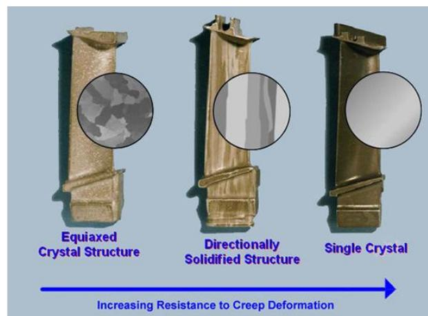
**Figure 5.7 :** *Different types of blades<sup>11</sup>*
