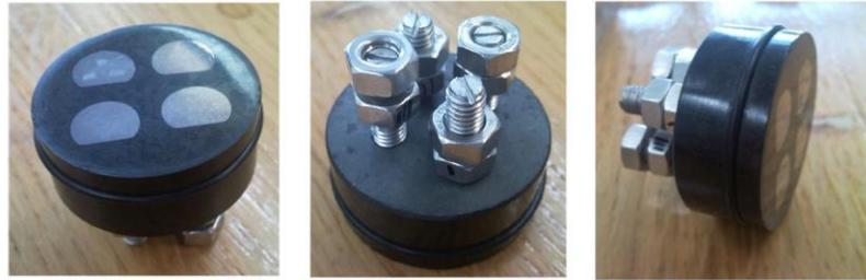
**Figure 5.10 :** Pictures of the CMSX-4 samples mounted into resin prepared for electropolishing by drilling holes on the backside in the resin upto the samples and bolt fixed for electric connections
