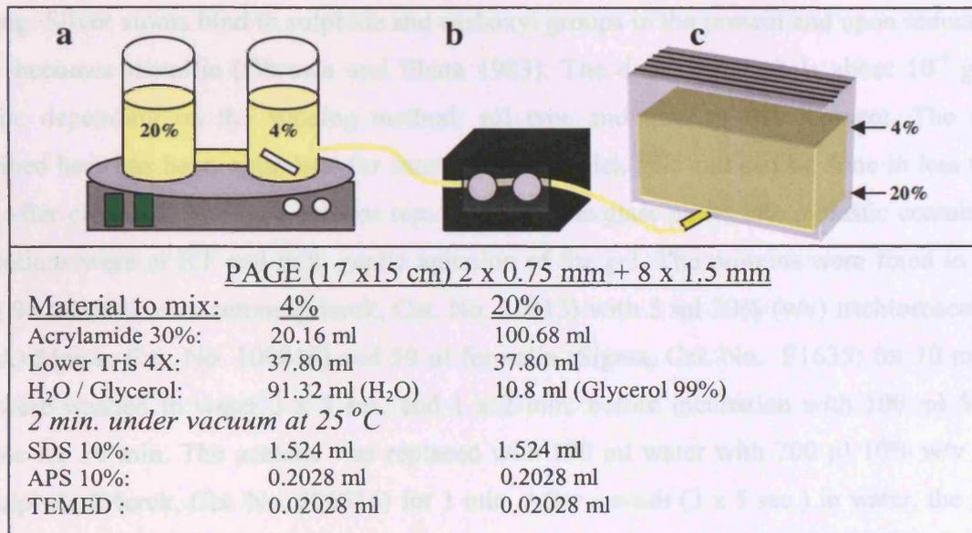
Figure 1. The equipment and the protocol for making gels. The left cylinder (a) contains the 20% acrylamide and the right cylinder the 4% acrylamide. The pump (b) moves the mixed solution to the multi gel chamber (c) so the first gel solution to enter will be 4% and the final drop will be 20%. By adjusting the content of acrylamide other gradients can be produced. The lower Tris buffer x4 contained 18.2% w/v Tris in dH<sub>2</sub>O, pH 8.9
