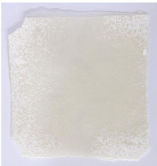
*Figure 5.15 Incomplete plasticisation of starch*
