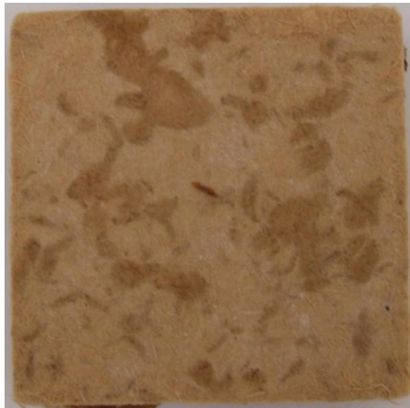
*Figure 5.19 Photograph of a fibreboard prepared using the method outlined in section 2.9.2, showing the mixing limitations of the method*
