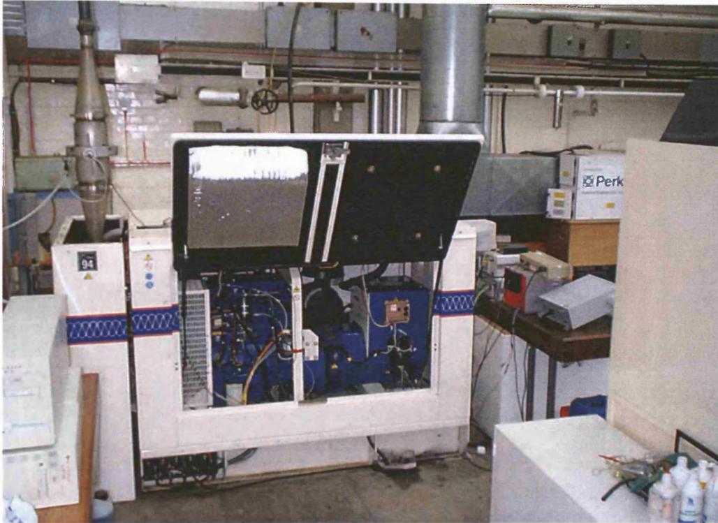
Picture 1. Diesel generator set test-bed installation in thermodynamics laboratory, showing the generator set, load bank and smoke detector.
