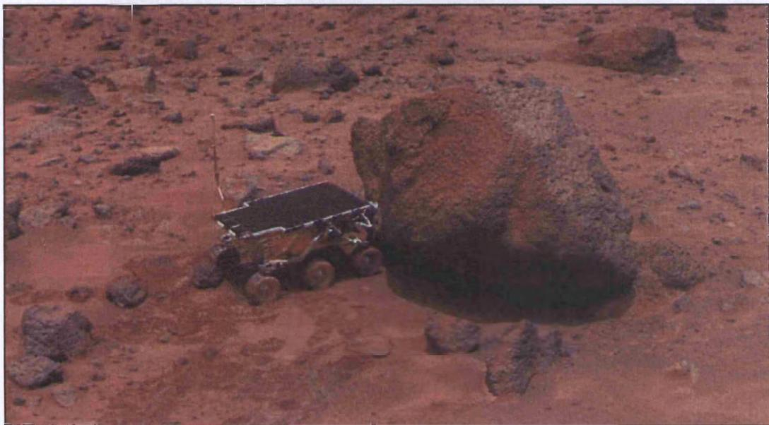
**Figure 2.10** The Sojourner rover on Mars with the APXS deployed by the ADM to analyse rock ‘Yogi’ (image courtesy of NASA).
