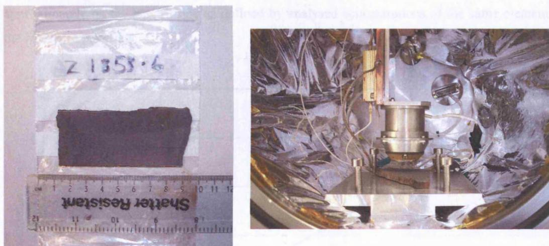
**Figure 7.1** (Left) Basalt rock slab (Z1853.6) of age 179 million years as determined by  $^{39}\text{Ar} \rightarrow ^{40}\text{Ar}$  radiometric dating. (Right) Experimental setup for measurement of a basalt slab in the calibration facility by the FS XRS.
