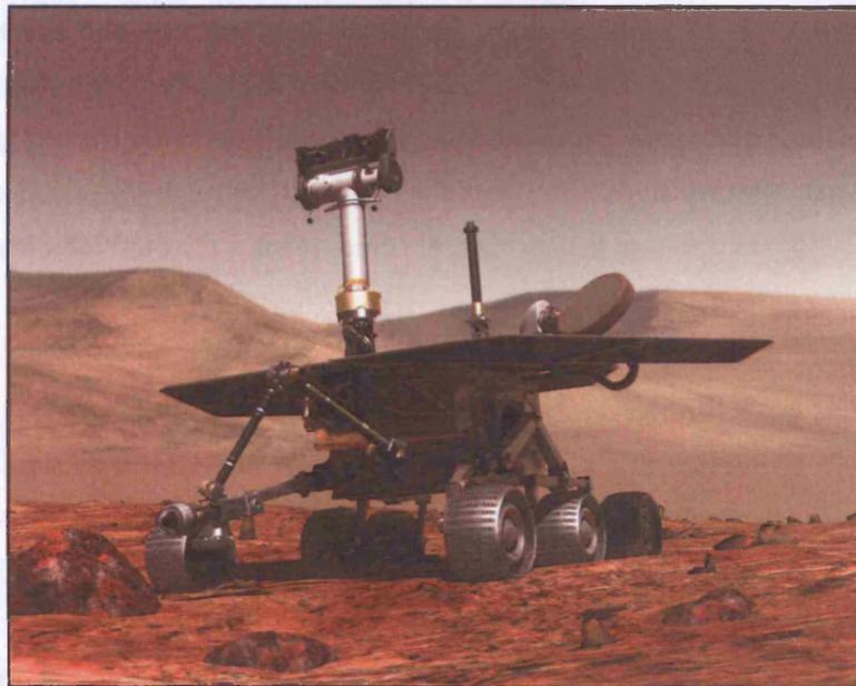
**Figure 2.11** Artist's impression of the Mars Exploration Rover with IDD deployed against a rock (image courtesy of NASA/JPL).
