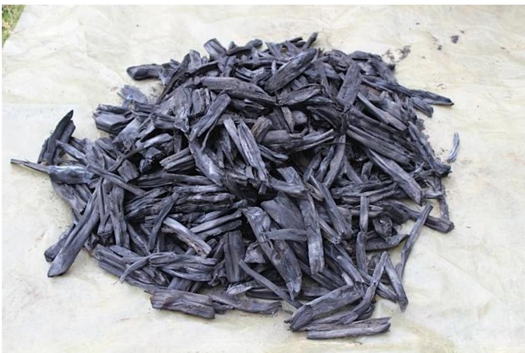
**Fig. 3.8.** Carbonized papyrus fines ready to be crushed and mixed with binding agent (photo: V. Lafford).
