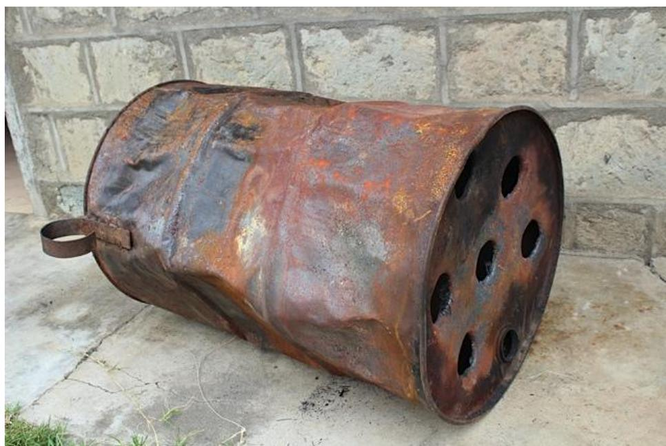
**Fig. 3.7.** Oil drum converted into a carbonizing kiln; holes in the base provide airflow (photo: V. Lafford).
