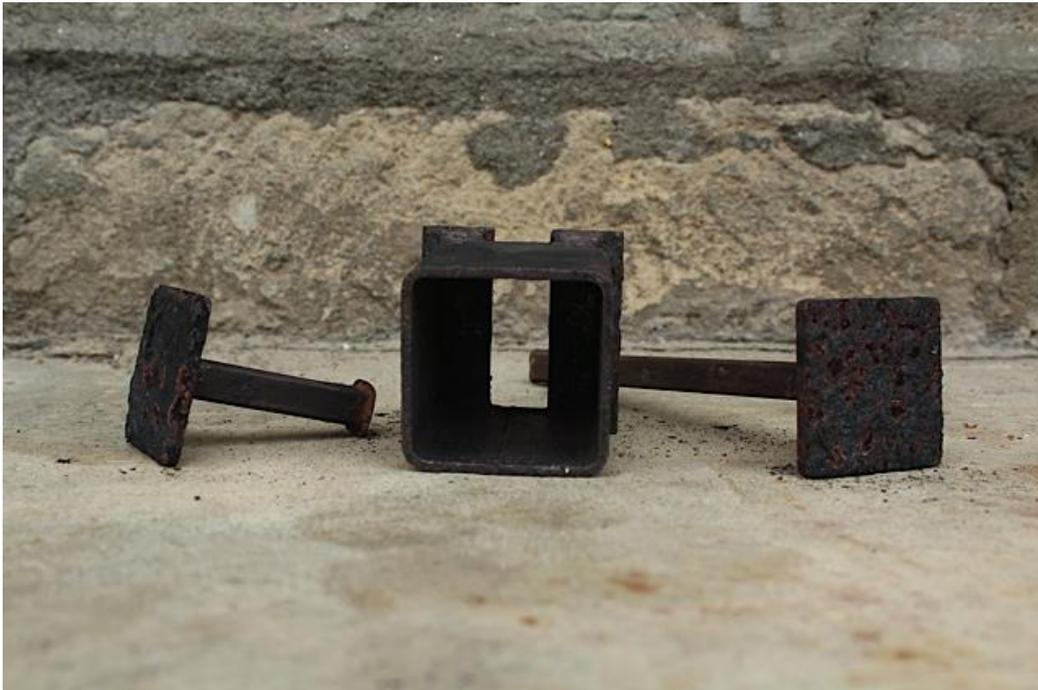
**Fig. 6.5.** Cuboid metal press (centre), with plunger (left) and ejector (right) (photo: V. Lafford).
