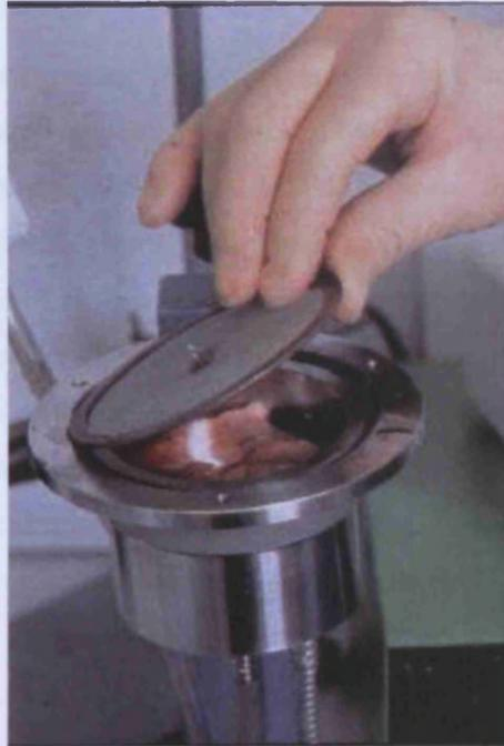
**Figure 7-3. Semi automated chamber for pancreatic digestion.**
