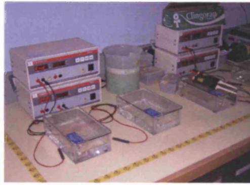
Figure 6-10. Gel electrophoresis used for PCR product analysis.
