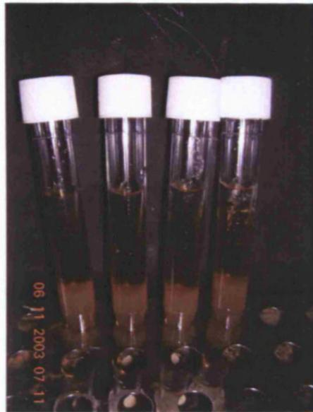
**Figure 6-5. Discontinuous BSA density gradients for rodent islet purification.**
