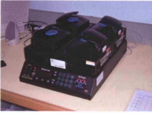
Figure 6-9. Thermocycler used for RT-PCR.
