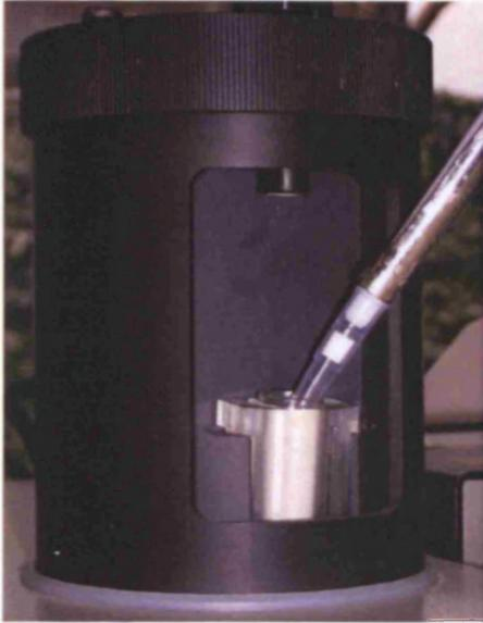
Figure 6-12. Luminometer cassette for ATP:ADP assay.
