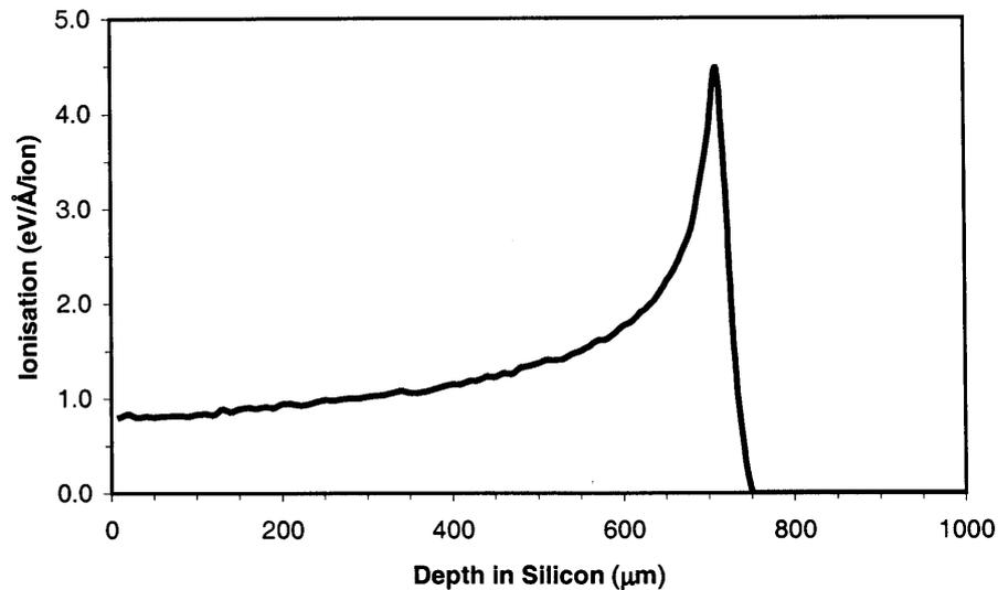
**Figure 3.11** The amount of ionisation caused by a 10 MeV proton in silicon modelled using SRIM 2003
