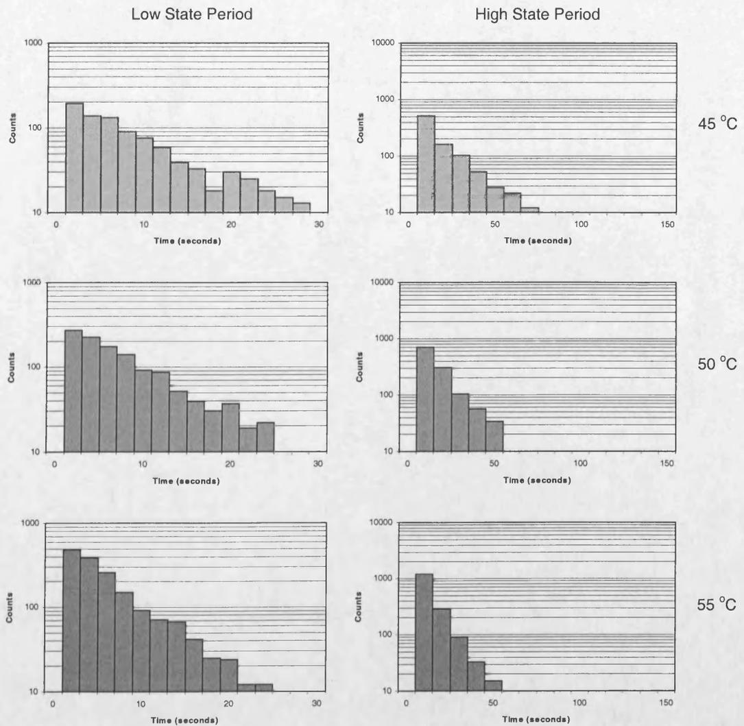
**Figure 6.19** Histograms of RTS high and low state periods from a sample of 8 RTS pixels at three temperatures
