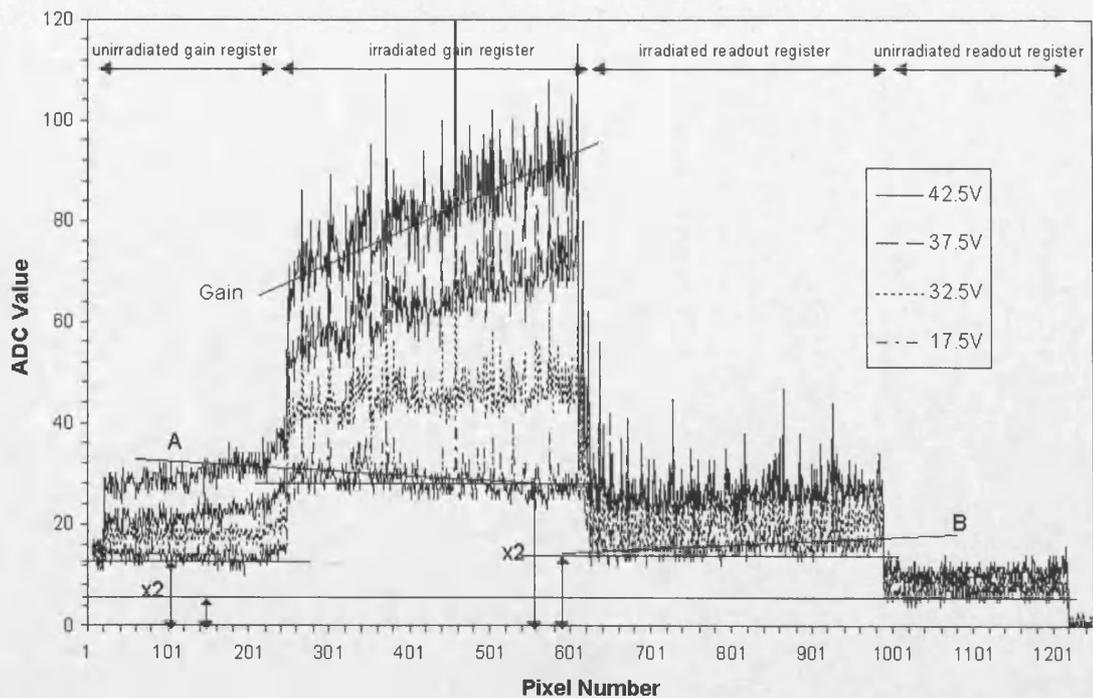
**Figure 4.9** The effect of different applied voltage on the L3Vision readout and gain registers. Slopes *A* and *B* show an indication of proton beam non-uniformity with low applied voltage. The gain is seen to increase sharply once the applied voltage is increased above 30 volts. The factor 2 increase in dark current level between the gain register and readout register due to different pixel sizes is also indicated
