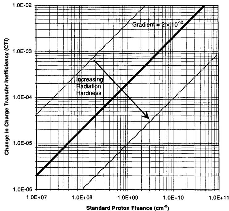
**Figure 3.20** A model for CTI growth variation with 10 MeV proton irradiation fluence for a CCD02 with an  $8\text{ }\mu\text{m}$  wide buried channel and  $22\text{ }\mu\text{m}^2$  pixels operating at  $-90\text{ }^{\circ}\text{C}$  (Holland et al. 1991)
