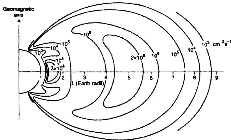
**Figure 3.3** A radial profile of the trapped electron flux in the Earth’s radiation belts for electrons of energy above 1 MeV (Daly 1989)
