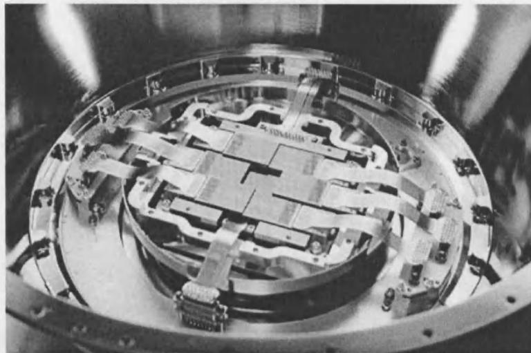
**Figure 5.2** The XMM-Newton EPIC MOS focal plane camera CCD arrangement
