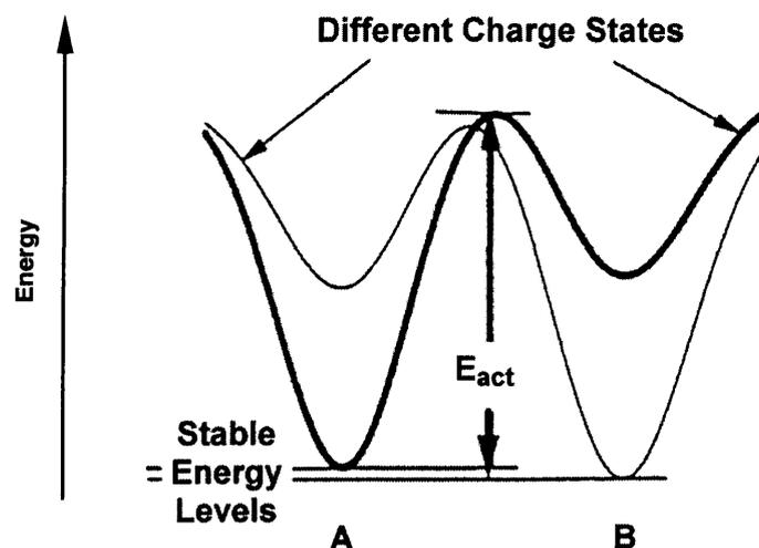
**Figure 6.23** Energy verses defect configuration for a defect with two stable states, A and B
