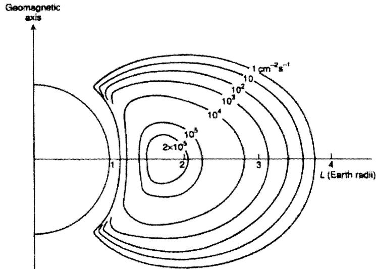
**Figure 3.4** A radial profile of the trapped proton flux in the Earth's radiation belts for protons of energy above 10 MeV (Daly 1989)
