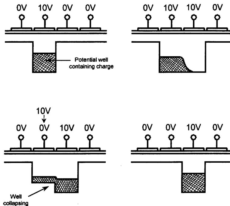
Figure 2.10 The charge transfer process
