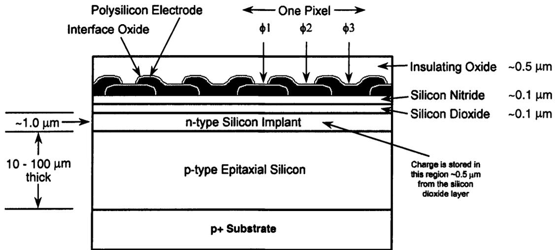
**Figure 2.4** A cross-section through a buried channel CCD showing the charge storage region that located away from the Si-SiO<sub>2</sub> interface
