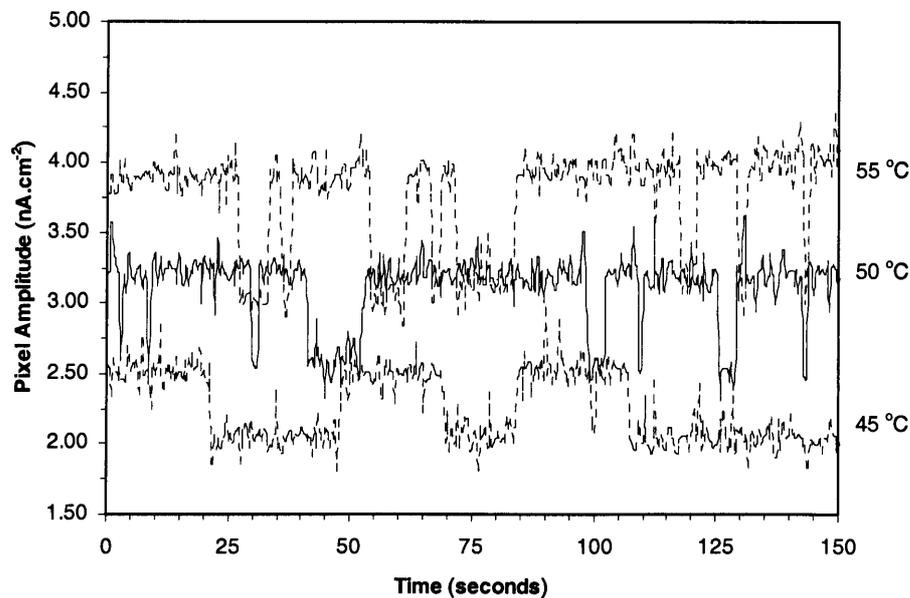
**Figure 6.18** The variation in high and low state period with temperature of an RTS pixel
