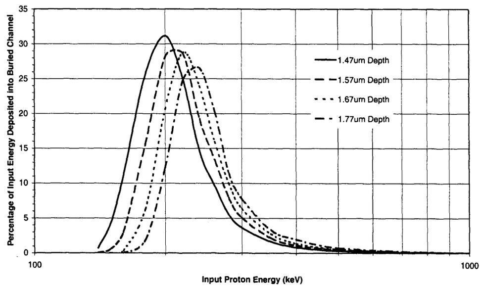
**Figure 5.10** The effect of varying buried channel width and depth below the CCD surface on the amount of energy deposited in the buried channel
