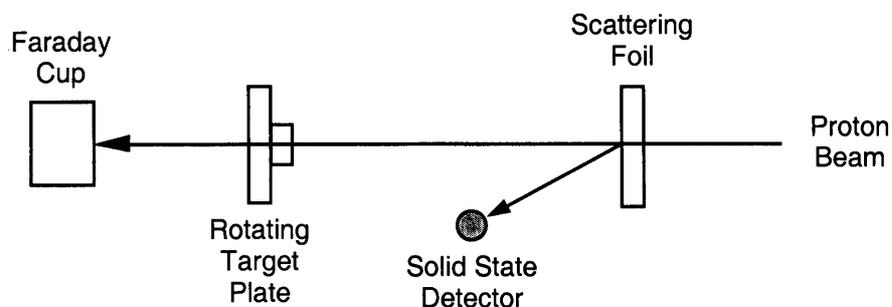
**Figure 6.2** A schematic of the Harwell tandem Van de Graaff beam line
