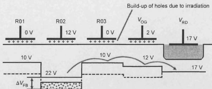
**Figure 3.15** The effect of oxide trapped charge on the potentials under the charge transfer electrodes and output structure of a CCD (adapted from Roy et al. 1989)
