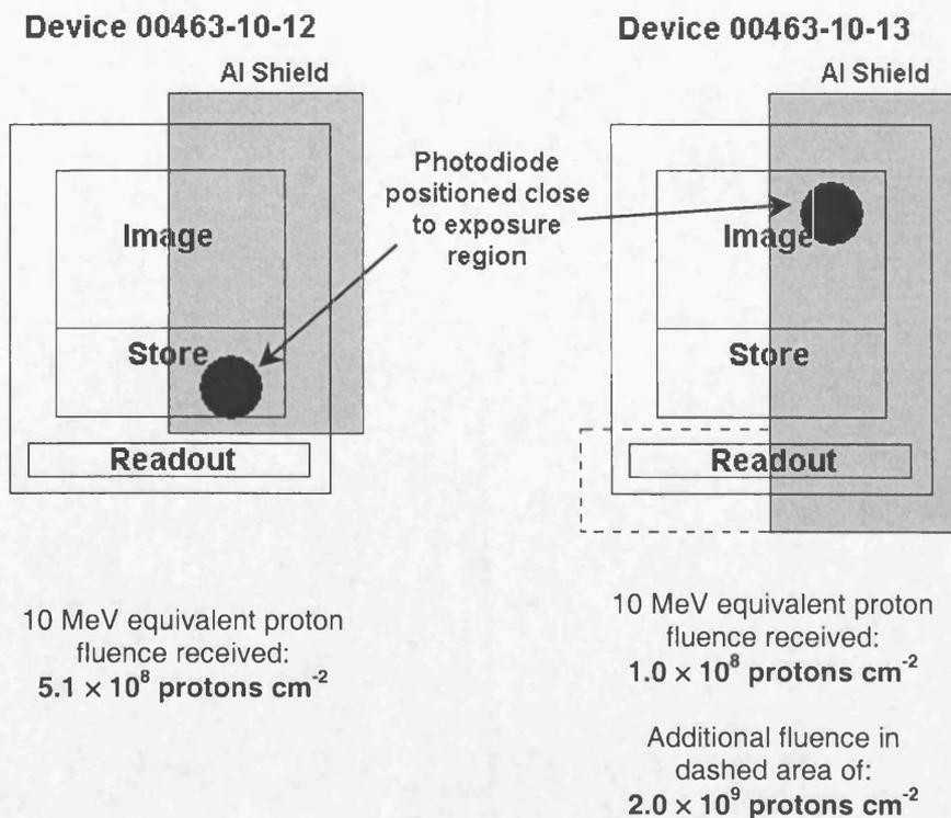
**Figure 4.7** A schematic showing the proton irradiated areas of two L3Vision CCD65 devices and the associated 10 MeV equivalent proton doses received
