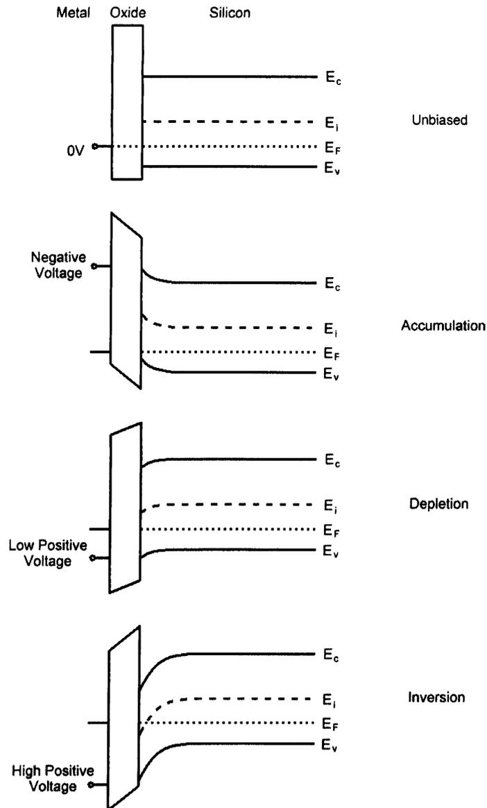
**Figure 2.6** The effect of electrode bias on the energy bands of the underlying silicon
