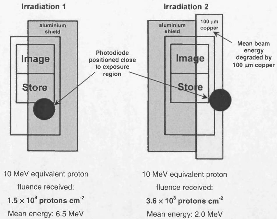
**Figure 6.1** A schematic showing the proton irradiated areas of device number 9211-5-3 and the associated 10 MeV equivalent proton doses received
