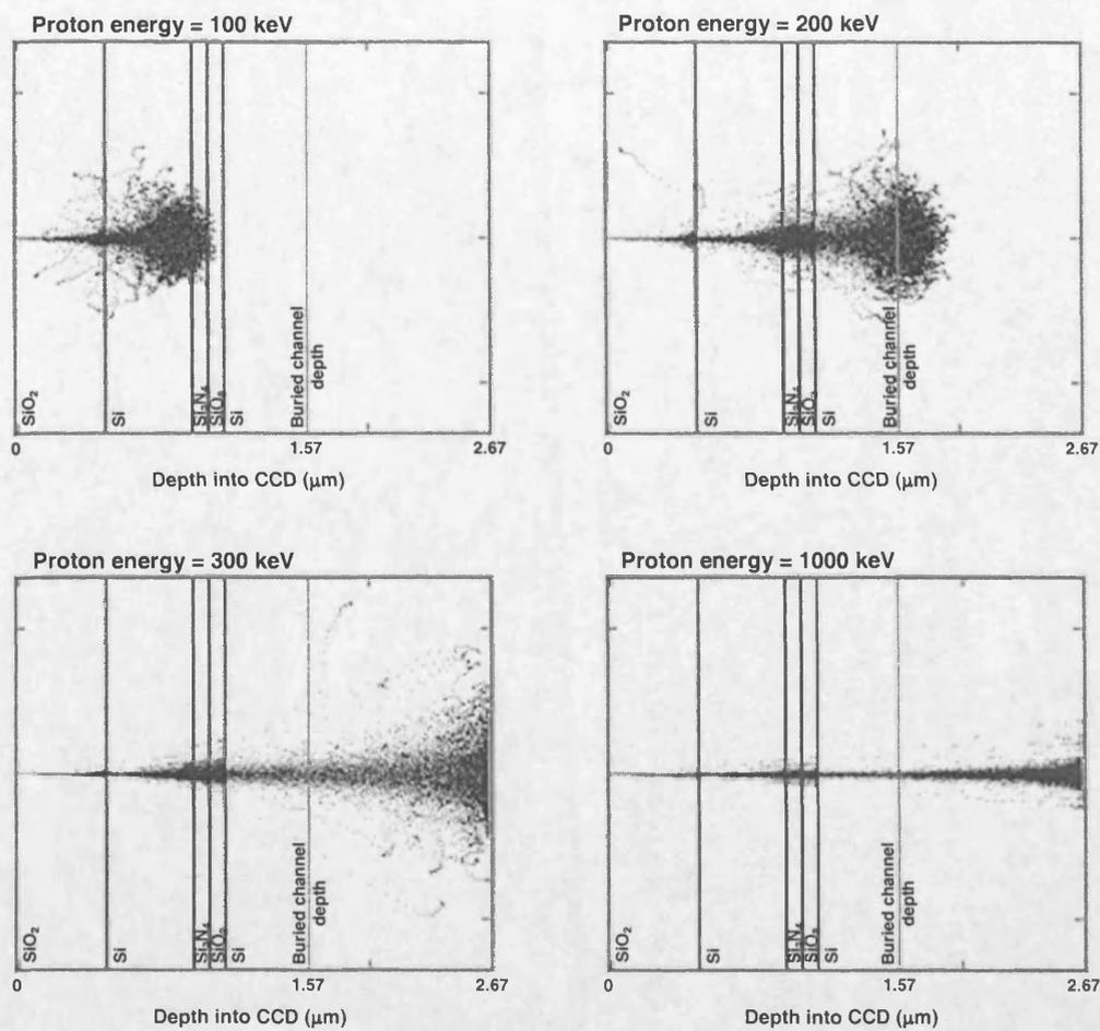
**Figure 5.8** The ionisation depth of protons interacting with a representative CCD22 structure over the charge transfer path. The buried channel depth is indicated in each panel, showing that protons of ~200 keV deposit the most energy into the buried channel volume
