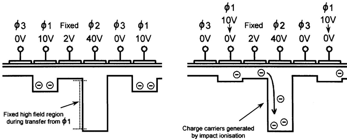
**Figure 4.2** Charge transfer in an L3Vision gain register
