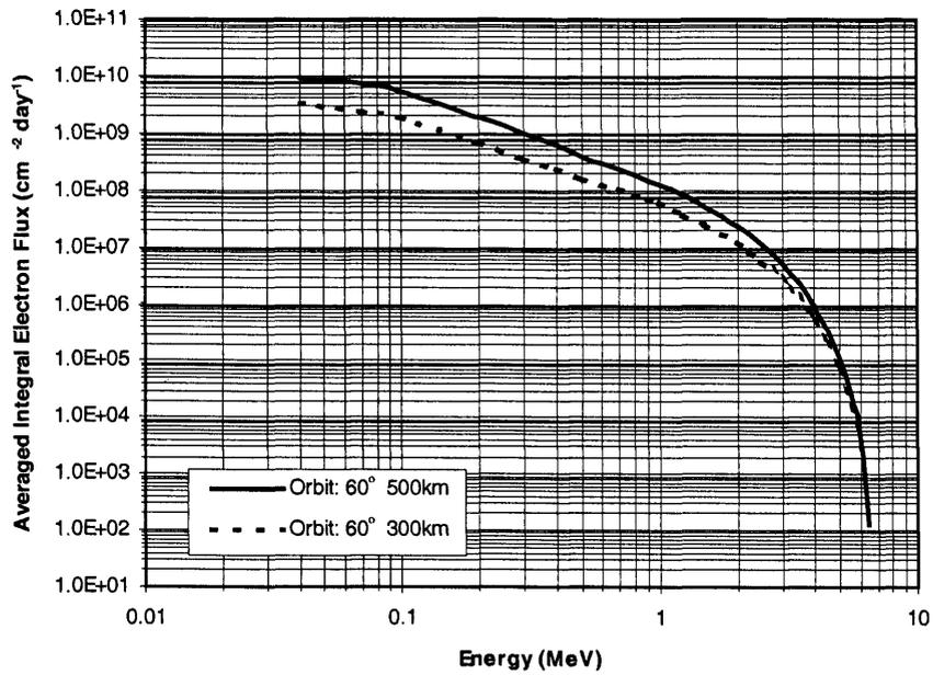
**Figure 3.5** Variation of the trapped electron flux with particle energy in the Earth's radiation belts modelled by AE8
