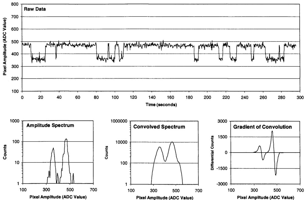
**Figure 6.9** Output from the RTS analysis software showing the sensitivity of the software to picking out the number of distinct amplitude levels present in the raw pixel amplitude data. The raw data was recorded with the CCD operating at 55 °C
