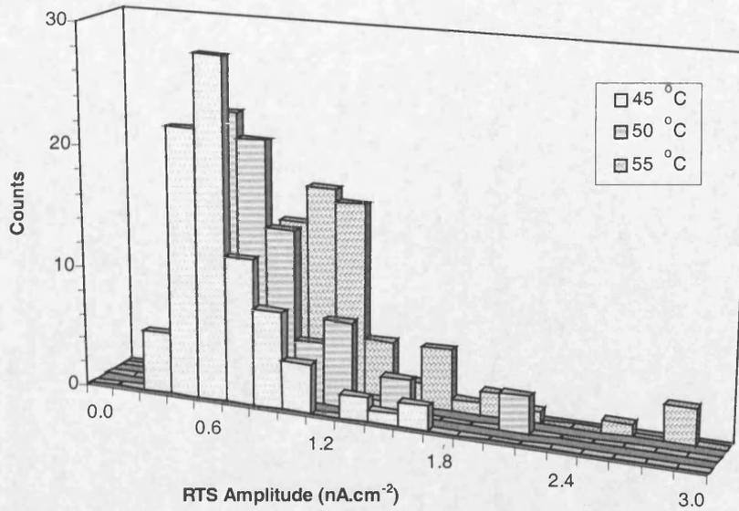
**Figure 6.14** Histograms of RTS transition amplitudes of 85 RTS pixels at three temperatures
