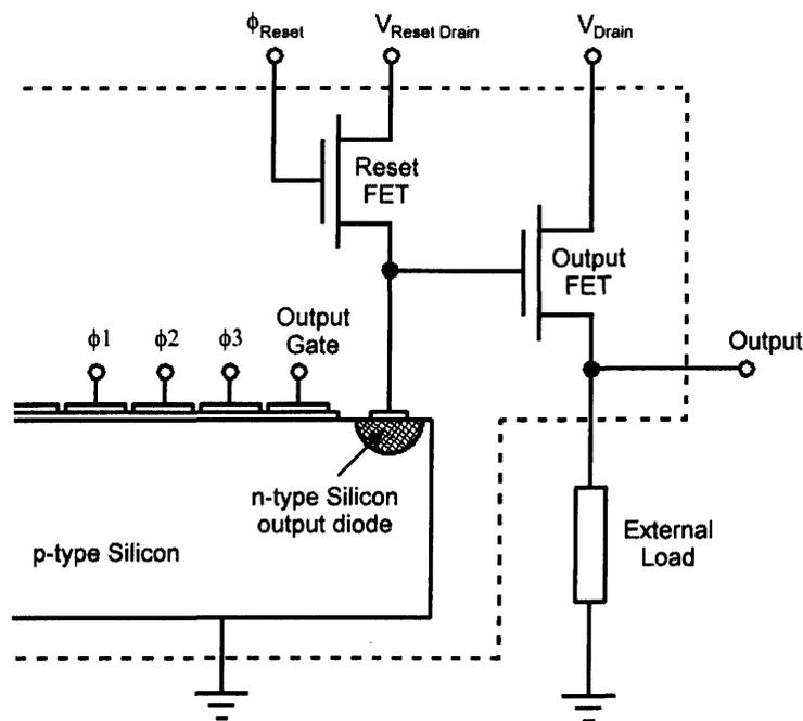
**Figure 2.12** A typical CCD readout register and output circuit
