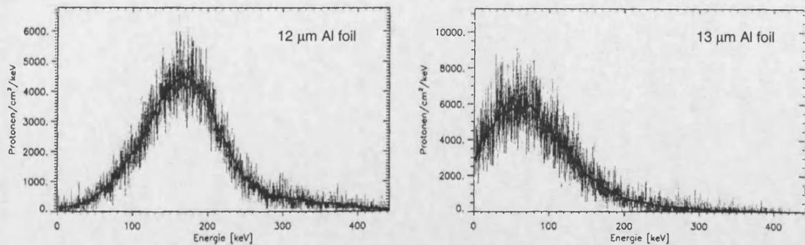
**Figure 5.4** Proton spectra measured by a pn-CCD using 12  $\mu\text{m}$  and 13  $\mu\text{m}$  Al foils (Clauß 2000)
