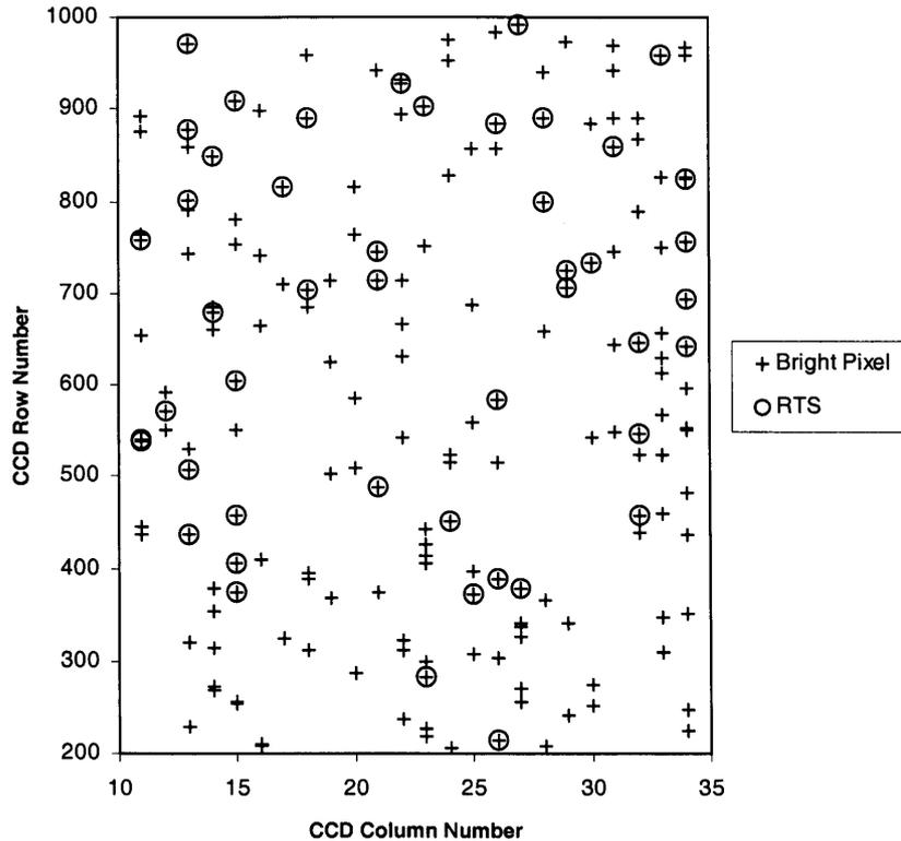
**Figure 6.5** The post-irradiation distribution of bright pixels and fluctuating pixels in device 9211-4-4
