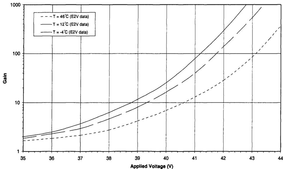
**Figure 4.3** E2V Technologies measured variation of gain with applied bias voltage for a CCD65
