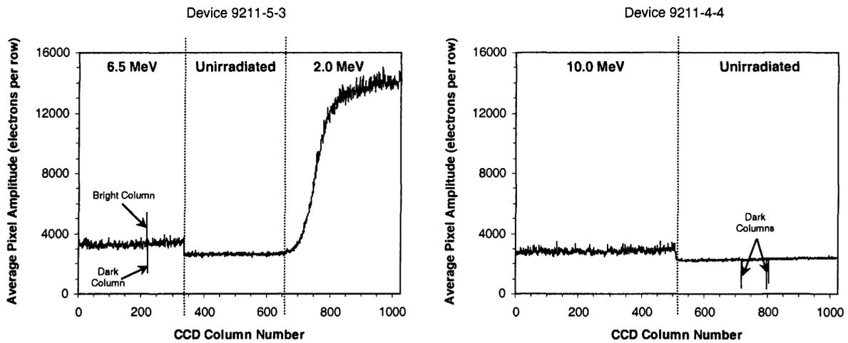
**Figure 6.4** Each graph shows the average pixel amplitude of 1000 rows in the image section of the proton-irradiated CCDs
