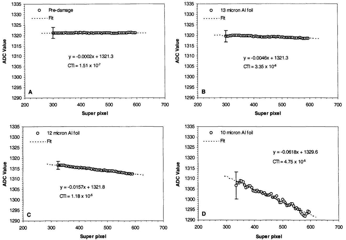
**Figure 5.9** The four panels depict the measured CTI before and after proton irradiation of device B5/21 through different thickness aluminium foils. The error bar in each panel is the same for each data point in that panel. Pixels have been binned in fives to create 'Super Pixels'
