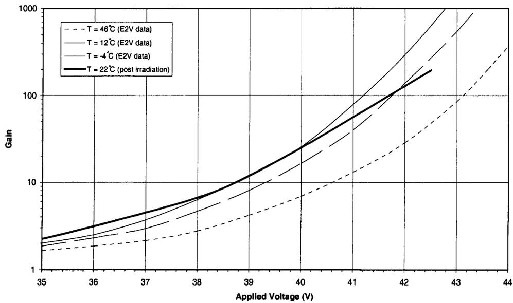
**Figure 4.10** Measured variation of gain with applied bias voltage post irradiation. Gain curves as measured by E2V Technologies for the L3Vision CCD65 are shown for comparison
