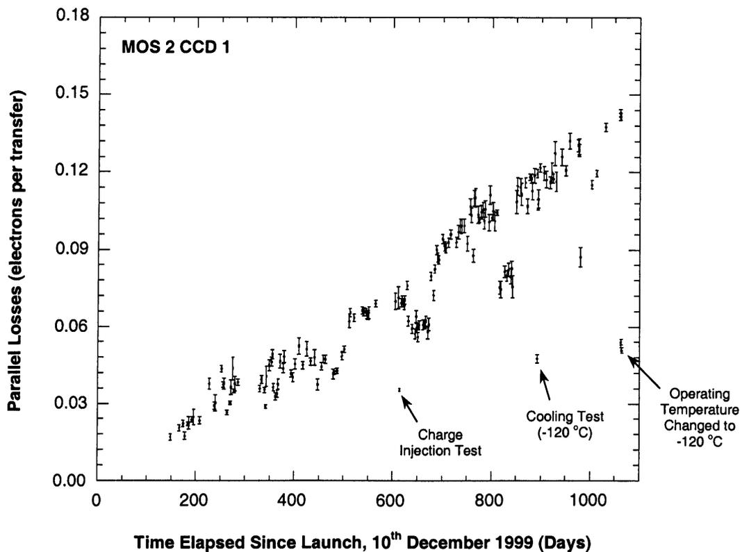
**Figure 5.11** On-orbit measurements of the Mn-K $\alpha$  parallel transfer losses of MOS 2 CCD 1 as a function of time
