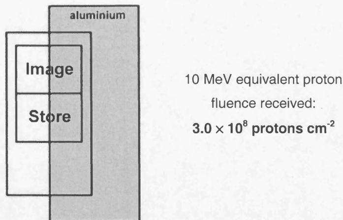
**Figure 6.3** A schematic showing the proton irradiated area of device number 9211-4-4 and the associated 10 MeV equivalent proton dose received
