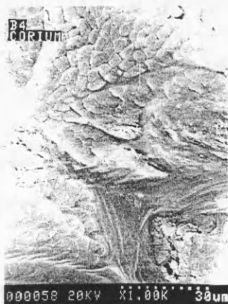
Figure 3.9. Scanning electron micrograph of leather treated with polyurethane, then plated (mag x 1000).
