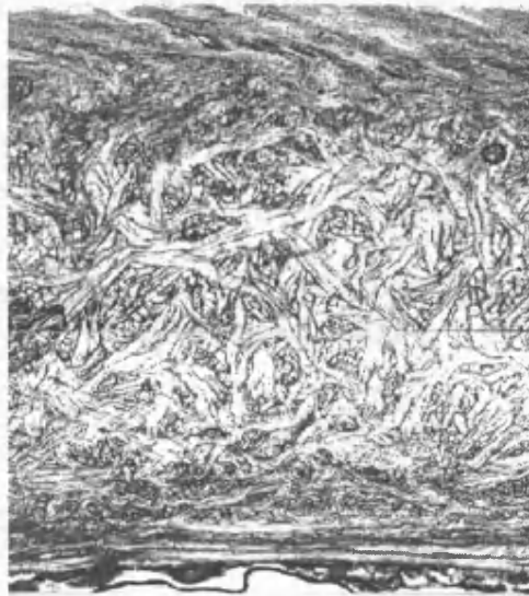
Figure 1.2. Photomicrograph illustrating the fibre structure of bovine skin.
