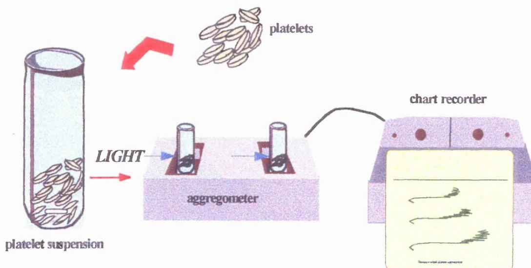
Figure 4.1 Aggregometer set up for platelet studies.
