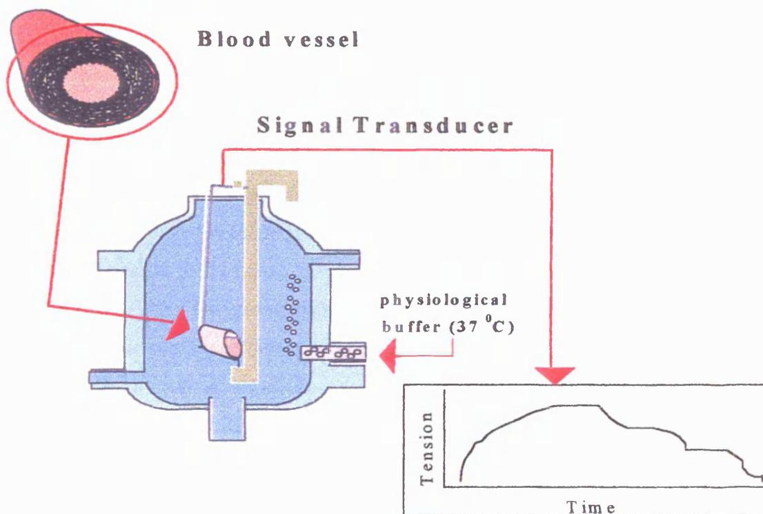
Figure 4.2 Organ chamber apparatus used for the measurement of vasorelaxation.
