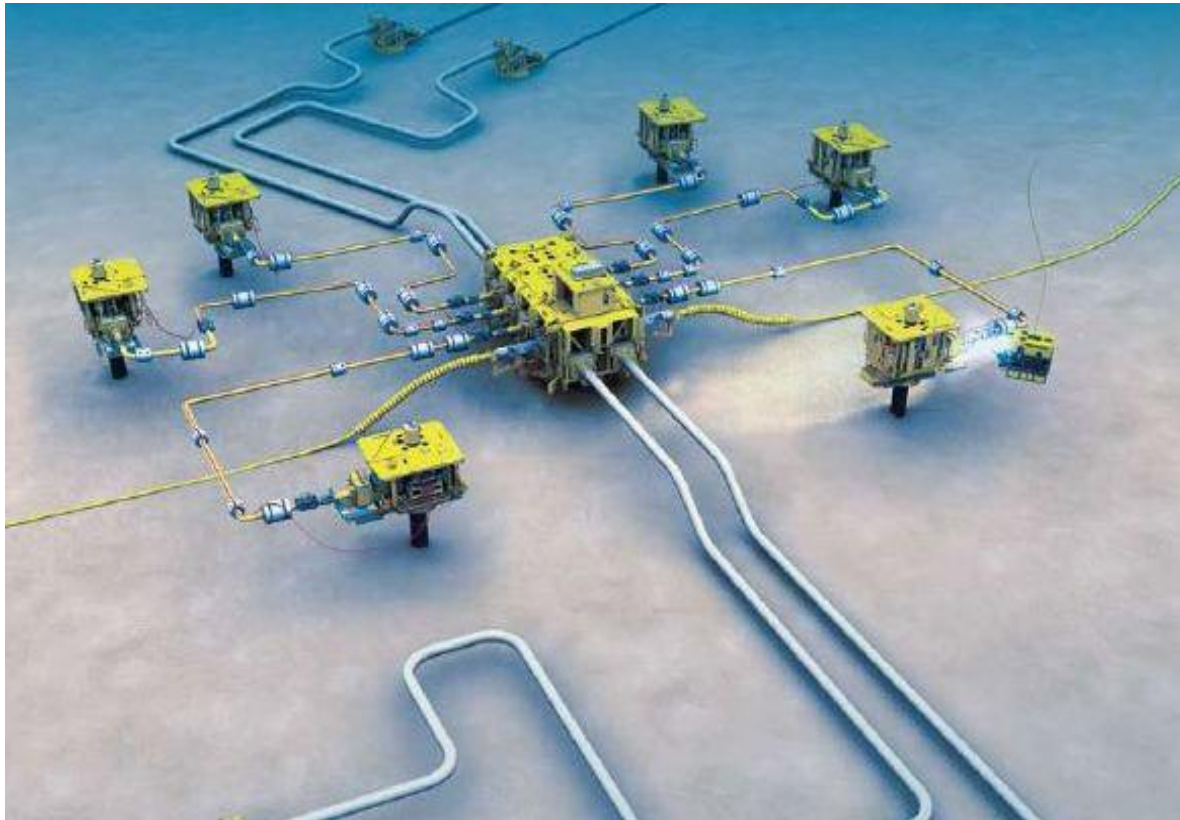
Figure 1-2 - Schematic of a subsea manifold surrounded by Christmas trees.
