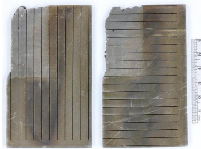
Figure 6-2 - Photographs of ED machined specimens prior to testing, together with scale bar (cm)
