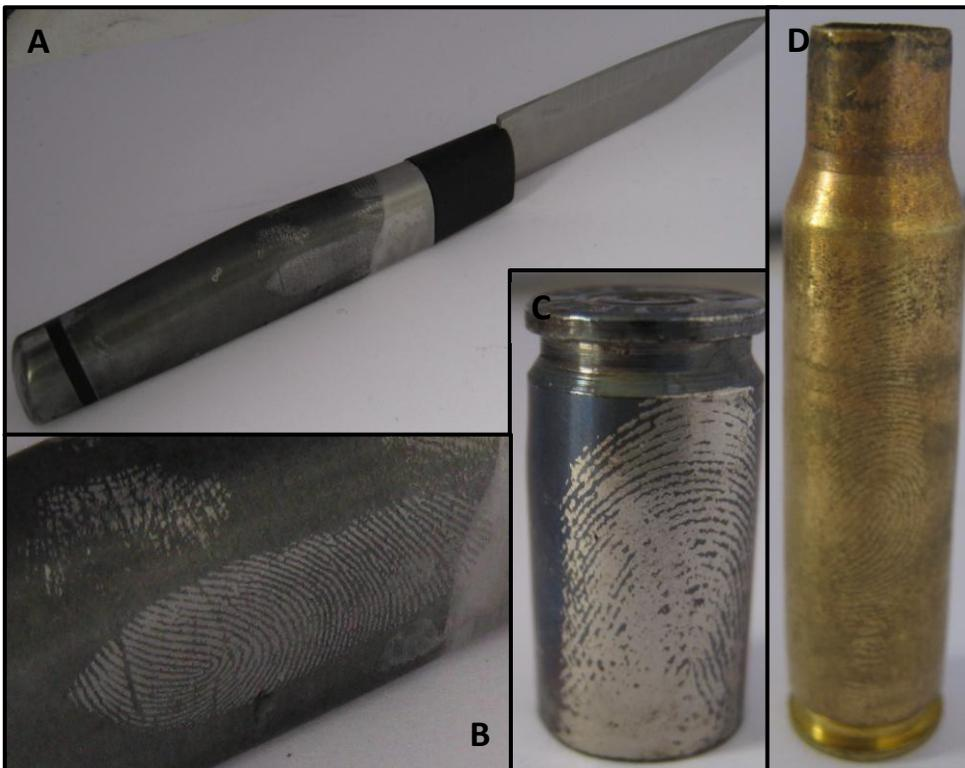
**Figure 3.45** P(Py-co-EDOT) 1:10 ratio enhanced fresh sebaceous fingerprints on (A + B) a stainless steel knife, (C) a Ni coated bullet casing and (D) a brass bullet casing.
