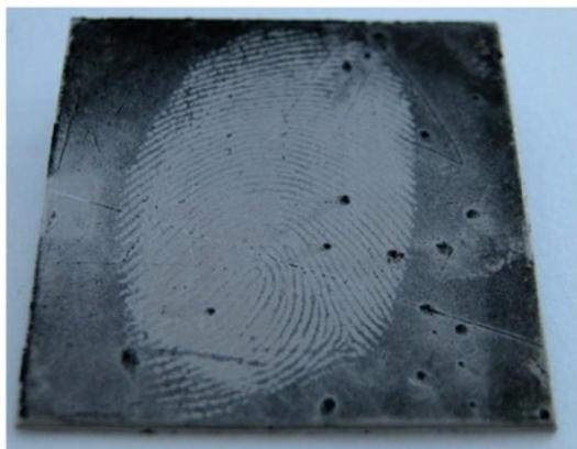
Fig. 2 Sebaceous fingerprint on stainless steel enhanced by PEDOT deposition from EDOT monomer solution containing  $1 \text{ mol dm}^{-3} \text{H}_2\text{SO}_4/0.01 \text{ mol dm}^{-3} \text{SLS}$ . Deposition (3500 s) on freshly fingerprinted stainless steel. Viewed *ex situ*; BAMLEY (C&D); GNUJIT: 3.
