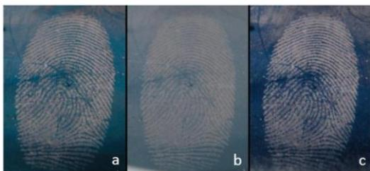
Fig. 3 Effect of pH on PEDOT enhancement for a sebaceous fingerprint on stainless steel (age 24 h under ambient conditions). Panel a: *ex situ*; panel b: *in situ* immersed in  $1 \text{ mol dm}^{-3} \text{H}_2\text{SO}_4$ ; panel c: *in situ* immersed in  $1 \text{ mol dm}^{-3} \text{KOH}$  (Bamley scale: grade 4).
