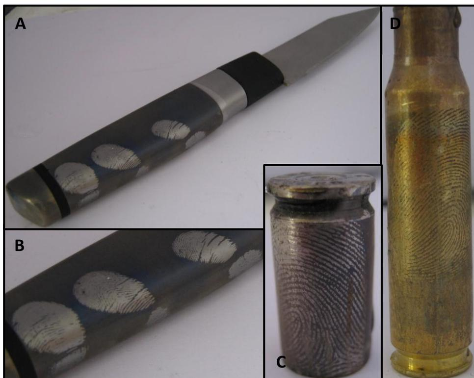
**Figure 3.46** P(Py-co-EDOT) 1:20 ratio enhanced fresh sebaceous fingerprints on (A + B) a stainless steel knife, (C) a Ni coated bullet casing and (D) a brass bullet casing.
