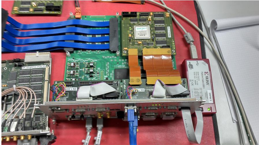
Figure 36: Photo of the DRPM motherboard
