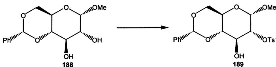
Methyl-4,6-*O*-benzylidene- $\alpha$ -D-glucopyranoside **188** (30.0 g, 0.11 mol), was dissolved in dry dichloromethane (300 ml). To this solution was added *N,N*-dimethyl-4-aminopyridine (2.6 g, 0.02 mol), and triethylamine (44 ml, 0.32 mol). This solution was cooled to 0°C
