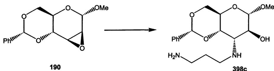
Methyl-2,3-anhydro-4,6-*O*- benzylidene- $\alpha$ -D-mannopyranoside **190** (788 mg, 2.98 mmol) and 1,3 diaminopropane (995  $\mu$ l, 11.92 mmol) was placed in a Youngs tube and stirred for
