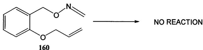
To the schrock catalyst **12b** (2 mol%) the oxime **160** (50 mg, 0.00026 mmol) was added. Nitrogen was bubbled through the flask as benzene (5 ml) was added. The reaction mixture was stirred at room temperature for 18h. The benzene was evaporated to yield a brown oil. TLC analysis showed only starting material to be present.
