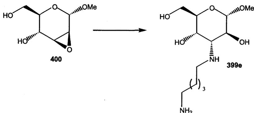
Methyl-2,3-anhydro- $\alpha$ -D-mannopyranoside **400** (230 mg, 1.31 mmol) and 1,5-diaminopentane (154  $\mu$ l, 1.31 mmol) was placed in a Youngs tube and stirred at 120<sup>o</sup>C for
