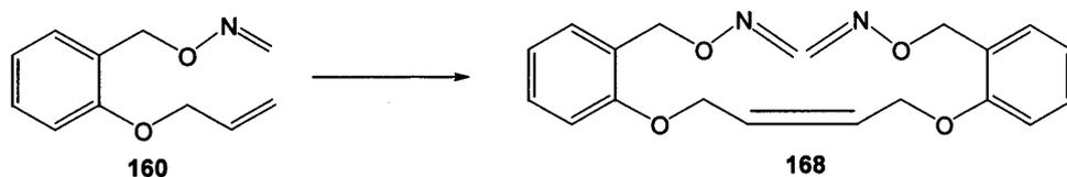
Under an atmosphere of nitrogen, oxime **160** (50 mg, 0.00026 mmol) was placed in a round bottom flask. Benzene (5 ml) was added and the mixture stirred under nitrogen for 3 mins. Catalyst **13b** (1.1 mol%) was added and the resulting mixture stirred at 60°C for 40h. The mixture was concentrated to yield a dark green oil. Chromatography on silica with petrol : diethyl ether (1:3) gave **168** (5 mg, 6%); *m/z* (ES) 377 (MH<sup>+</sup>Na)
