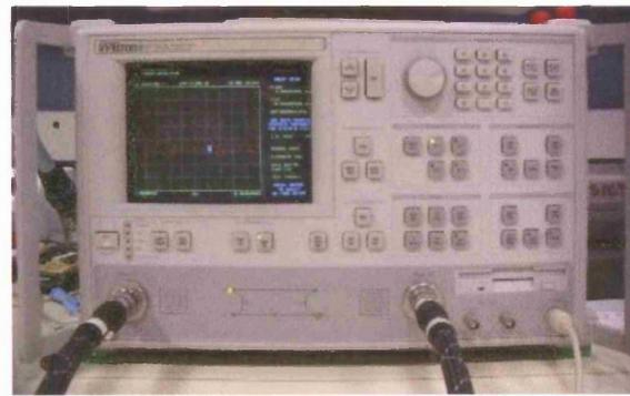
**Figure 5.** The Vector Network Analyser.
