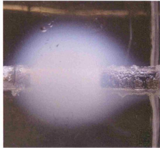
**Figures 2.12 and 2.13.** Figure 2.12 (to the left) shows a direct launch MEA applicator radiating into PAG temperature sensitive gel. The spherical field radiated from the end of the applicator can be appreciated. Figure 2.13 to the right shows a modified MEA applicator in which the cutting tip has been introduced. It can be appreciated that the field is centred more proximally along the applicator shaft rather than being emitted from the distal cutting tip.
