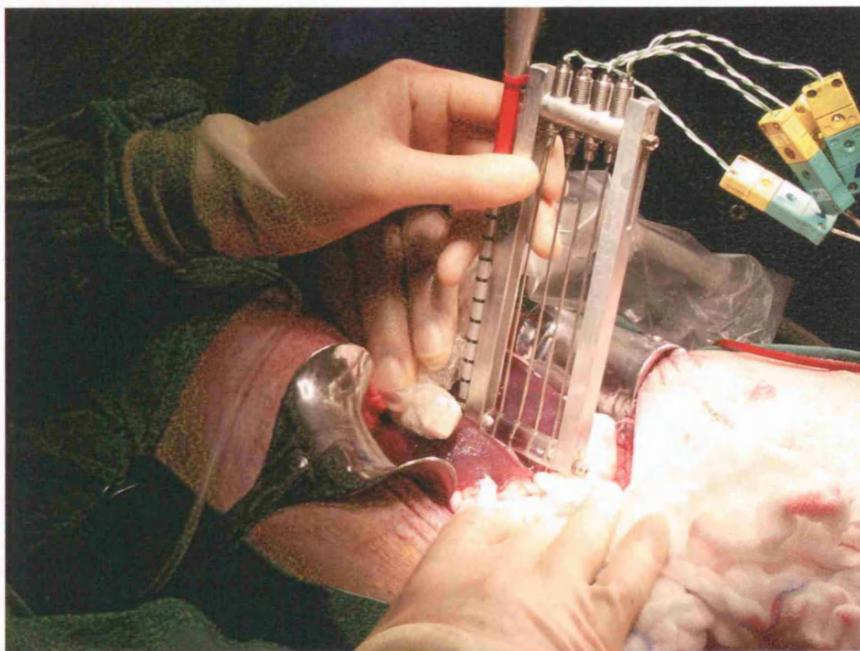
**Figure 3.1:** The microwave applicator (red sleeve) is being placed into a piece of porcine liver parenchyma. The aluminium jig seen contains thermocouples used for
