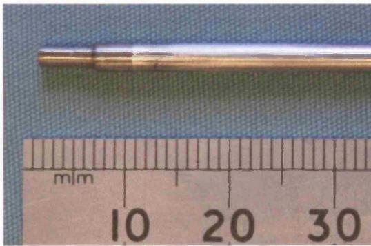
**Figure 4.** The open-ended coaxial probe used for taking permittivity readings.
