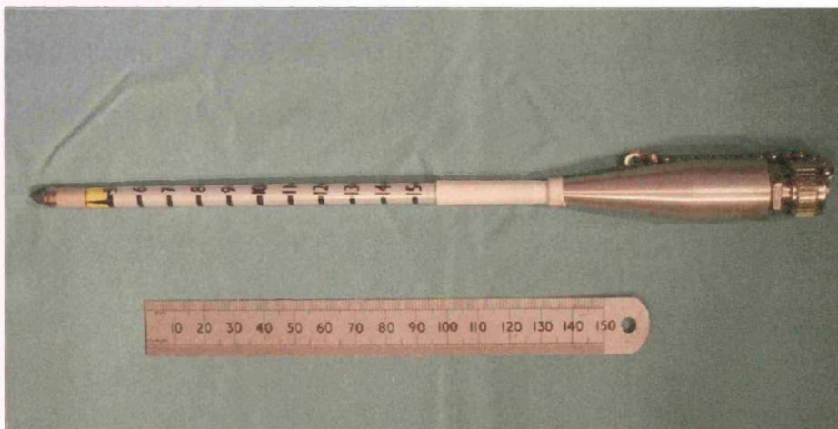
**Figure 2.14.** 2.45GHz interstitial microwave applicator.
