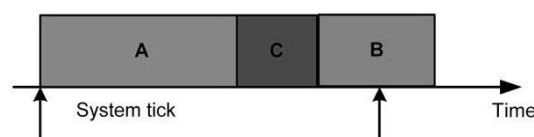
Figure 2: Illustration of overall change in system behaviour if the execution time of task A takes longer than expected
